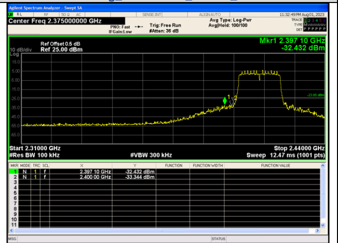
Out Of Band Emission IEEE 802.11n_Channel 1_20MHz_Antenna 1
