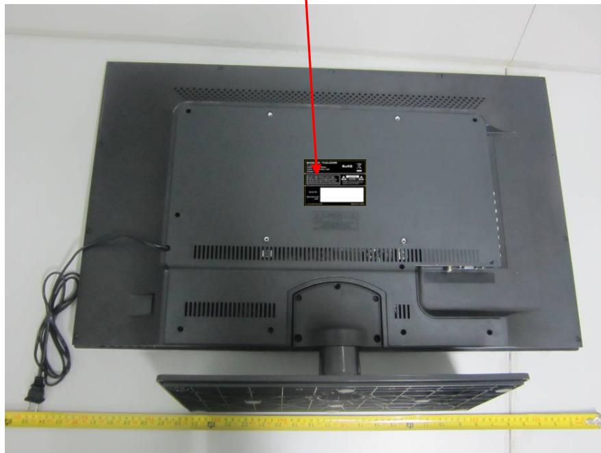
The label shown shall be permanently affixed at a conspicuous location on the device and be readily visible to the user at the time of purchase (Labeling requirements per 2.925)
