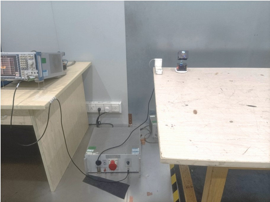
Conducted Emission Test Setup
