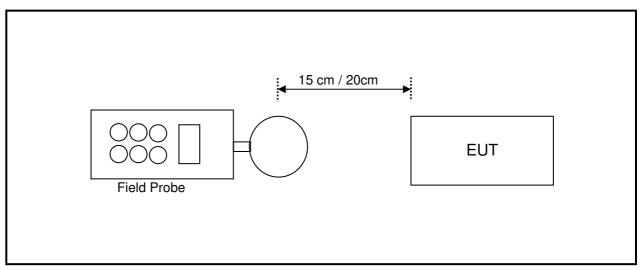
Note: Measurements should be made from all sides and the top of the primary/client pair, with the 15 cm or 20 cm measured from the center of the probe(s) to the edge of the device.
