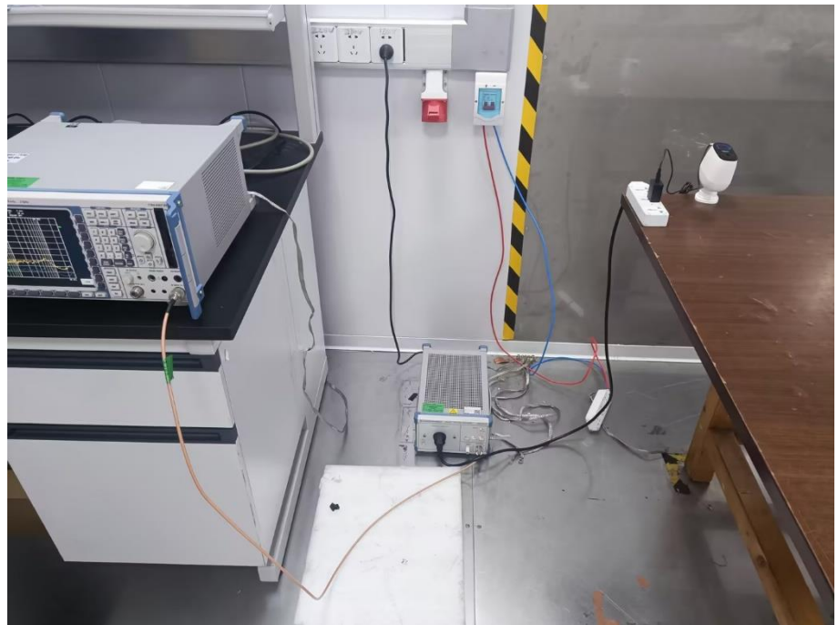
Conducted Emission Test Setup
