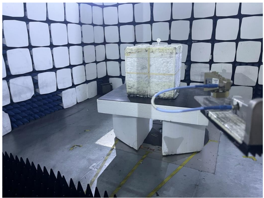
Radiation Emission Test Setup (Above 18GHz)
