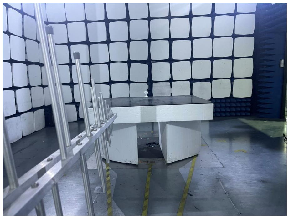
Radiation Emission Test Setup (30MHz to 1GHz)
