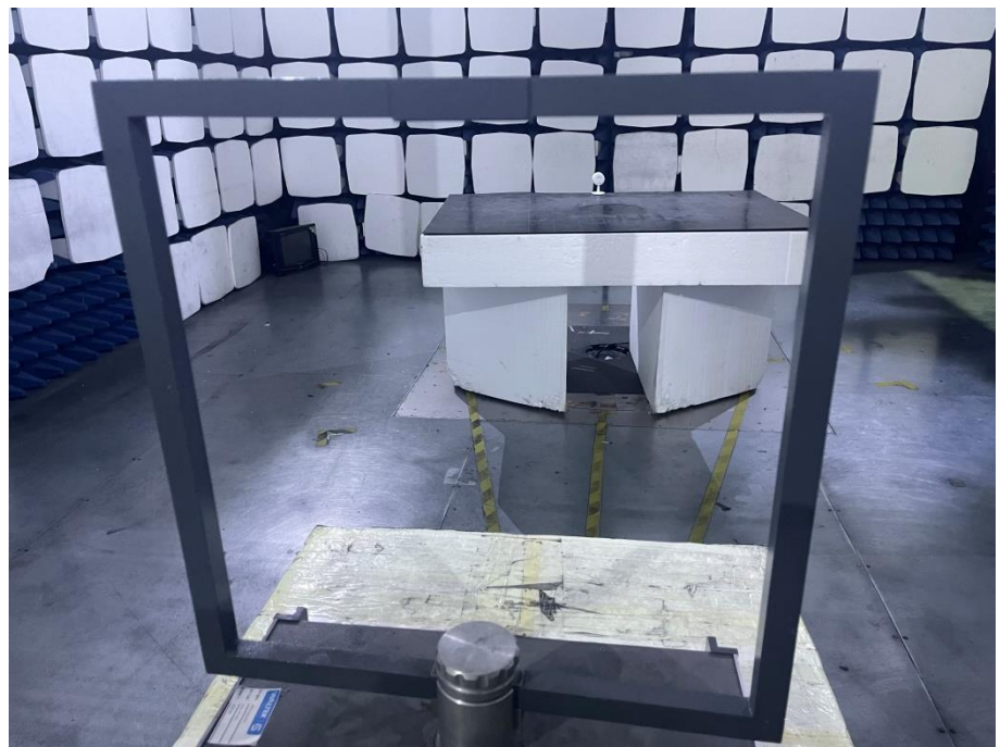
Radiation Emission Test Setup (Below 30MHz)
