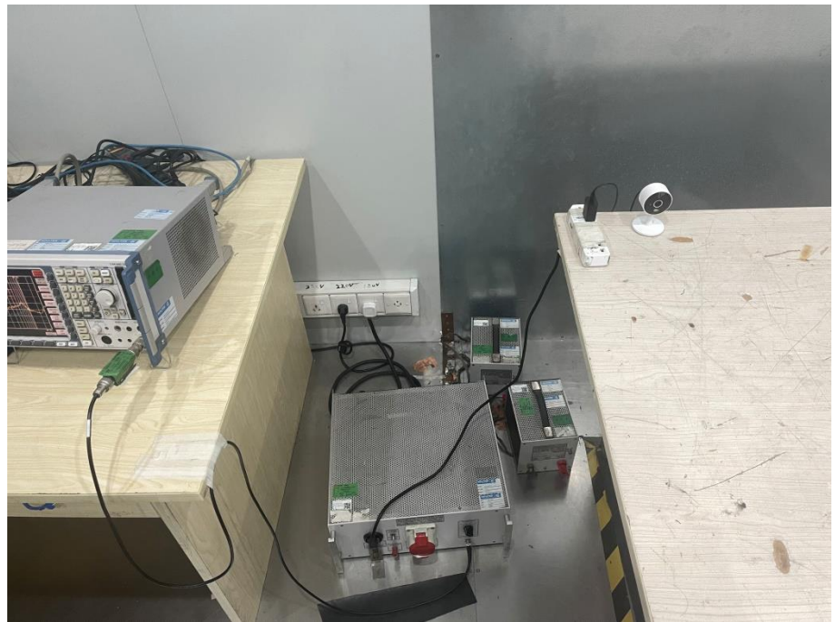
Conducted Emission Test Setup
