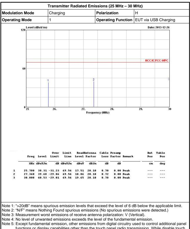
functions or display capabilities other than the touch panel radio transmission. While disable touch panel radio transmission, other emissions have the same levels. Therefore other emissions level could be exceed the fundamental emission level.
