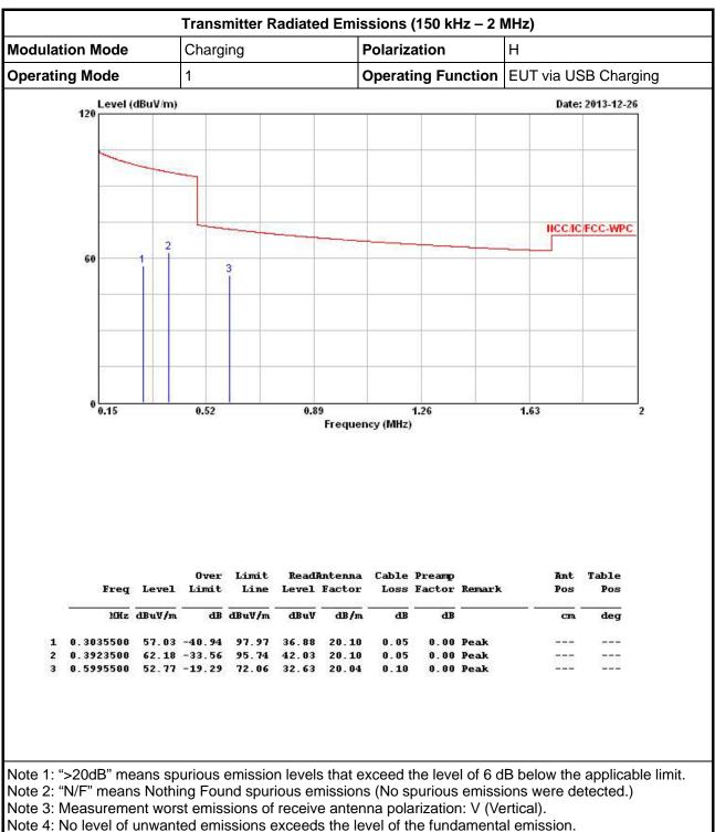
Note 5: Except fundamental emissions other emissions from digital circuitry used to control additional panel functions or display capabilities other than the touch panel radio transmission. While disable touch panel radio transmission, other emissions have the same levels. Therefore other emissions level could be exceed the fundamental emission level.
