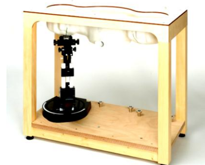
Fig 5.3 Photo of SAM Phantom
