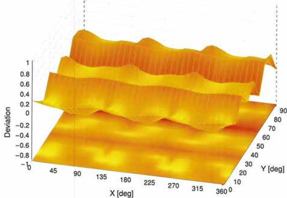
60GHz: 3D isotropy, E-field parallel to probe axis
