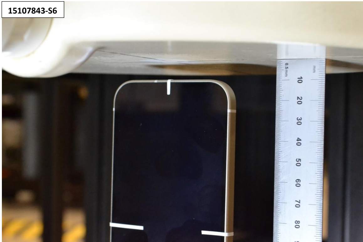
Photograph 17: Hotspot, Edge Bottom, 10 mm
