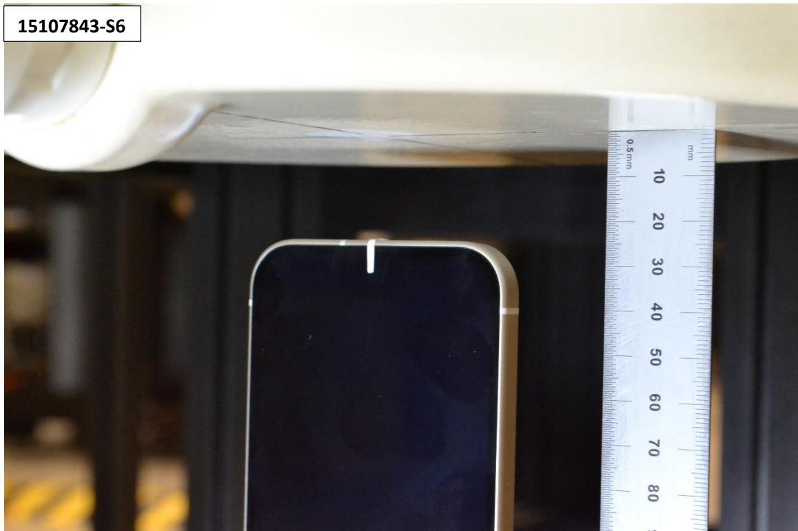
Photograph 18: Hotspot, Edge Bottom, 25 mm
