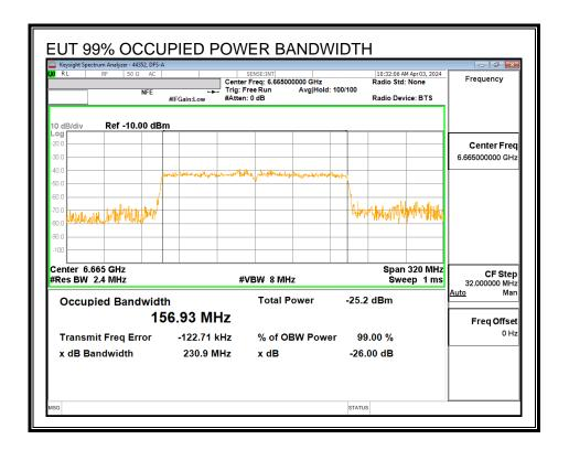
The manufacturer has declared that the 99% Occupied Channel Bandwidth is 157.94 MHz.
