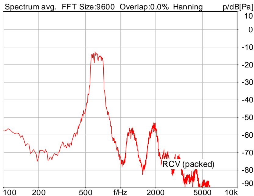
Distortion (Noise) RCV (packed): 31.45 dB (2.68%) Ok
