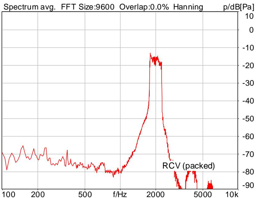
Distortion (Noise) RCV (packed): 32.89 dB (2.27%) Ok
