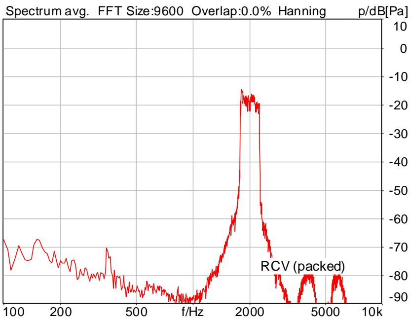
Distortion (Noise) RCV (packed): 40.42 dB (0.95%) Ok
