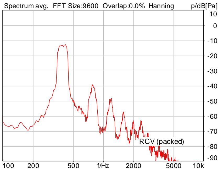
Distortion (Noise) RCV (packed): 26.52 dB (4.72%) Ok
