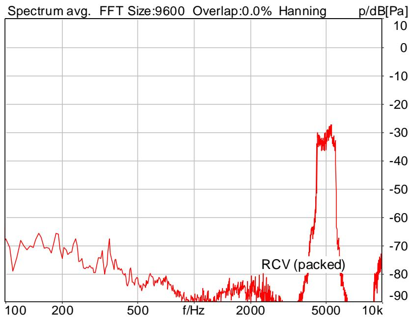
Distortion (Noise) RCV (packed): 33.62 dB (2.09%) Ok
