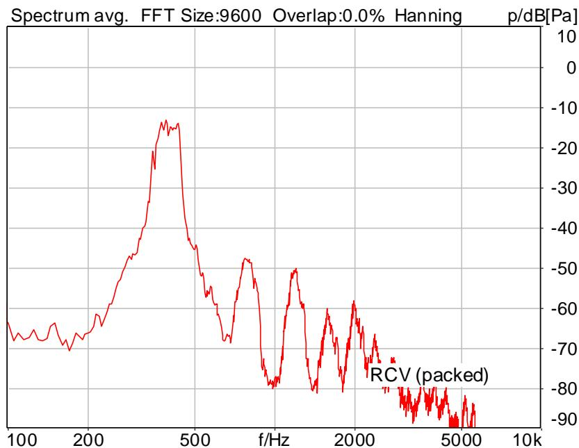
Distortion (Noise) RCV (packed): 29.21 dB (3.46%) Ok
