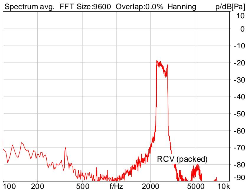
Distortion (Noise) RCV (packed): 41.86 dB (0.81%) Ok
