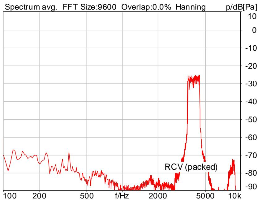
Distortion (Noise) RCV (packed): 34.90 dB (1.80%) Ok
