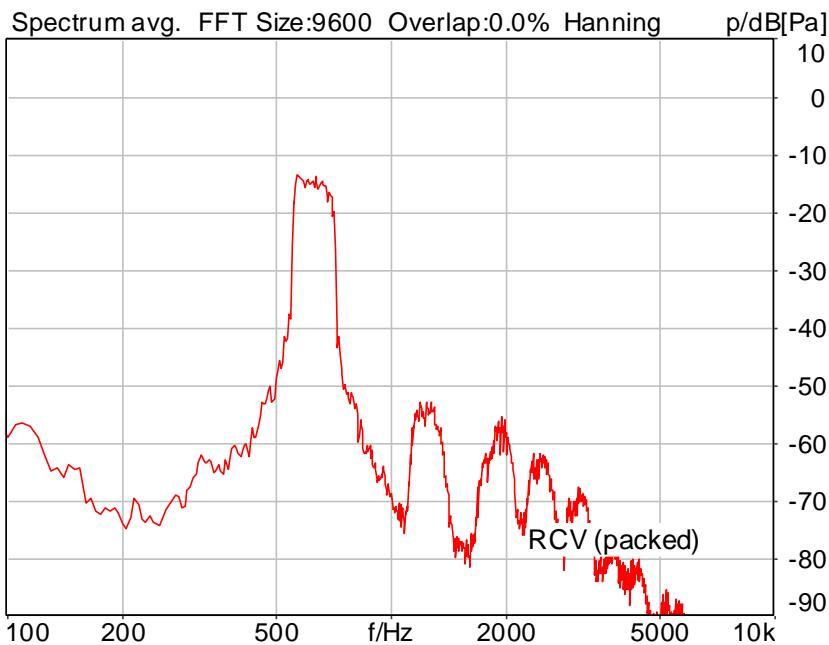
Distortion (Noise) RCV (packed): 32.74 dB (2.31%) Ok
