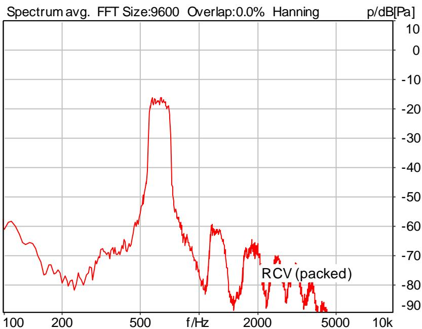
Distortion (Noise) RCV (packed): 37.11 dB (1.40%) Ok
