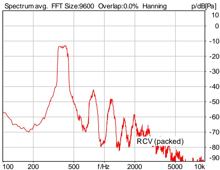
Distortion (Noise) RCV (packed): 28.69 dB (3.68%) Ok
