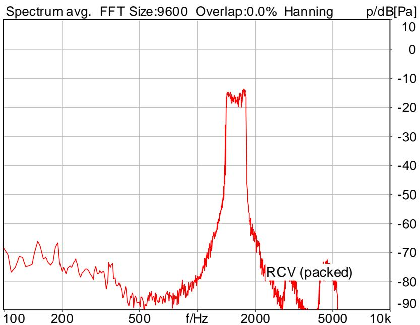
Distortion (Noise) RCV (packed): 40.58 dB (0.94%) Ok
