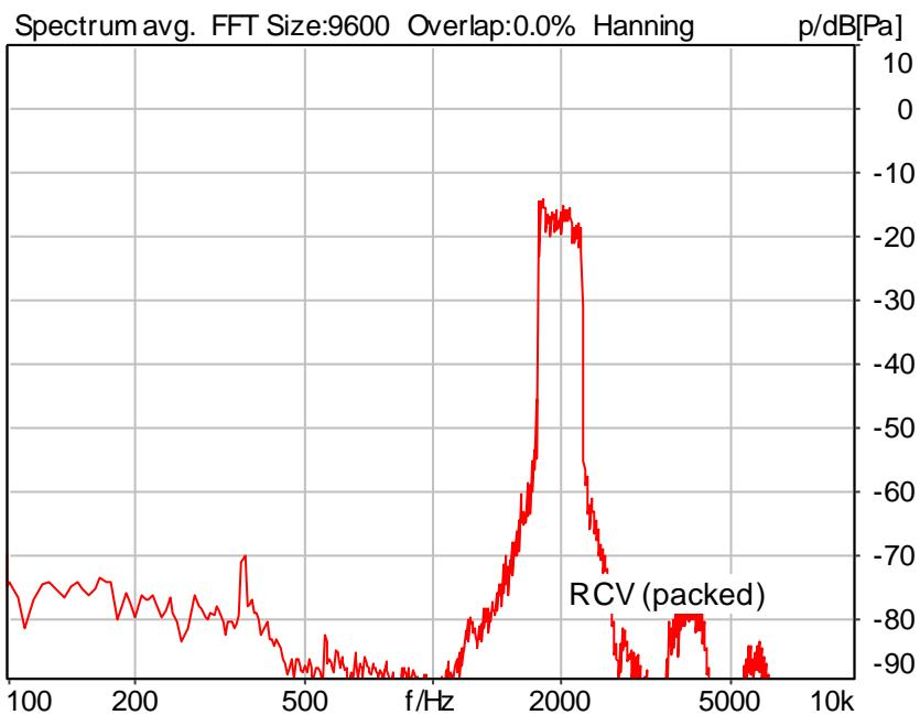
Distortion (Noise) RCV (packed): 43.67 dB (0.66%) Ok
