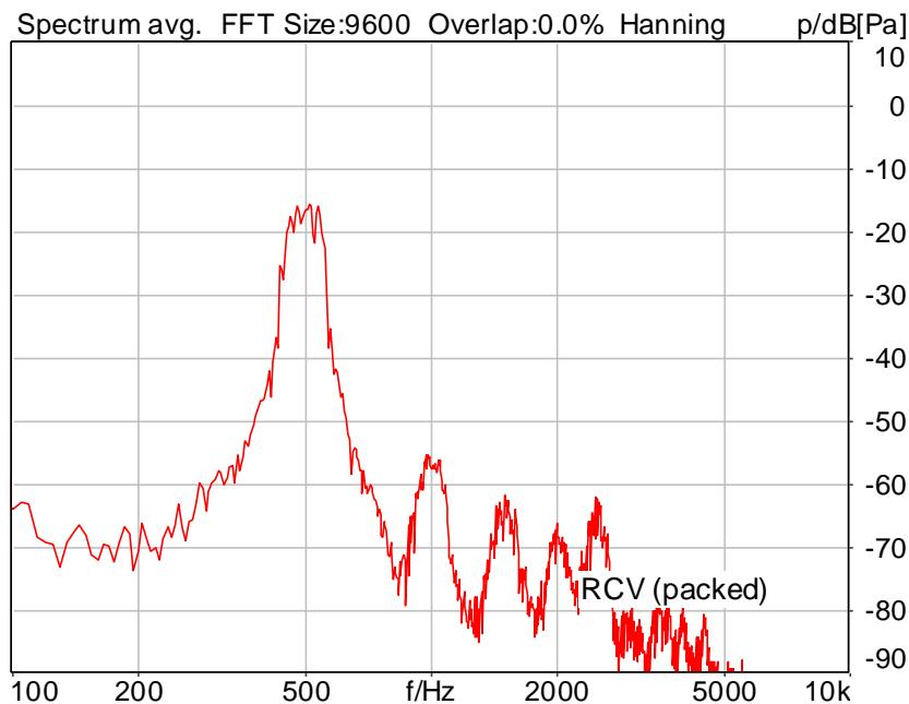
Distortion (Noise) RCV (packed): 31.44 dB (2.68%) Ok
