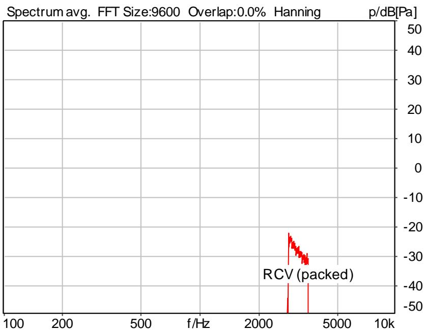
Distortion (Noise) RCV (packed): 42.29 dB (0.77%) Ok
