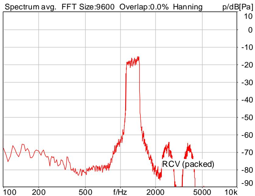
Distortion (Noise) RCV (packed): 30.84 dB (2.87%) Ok
