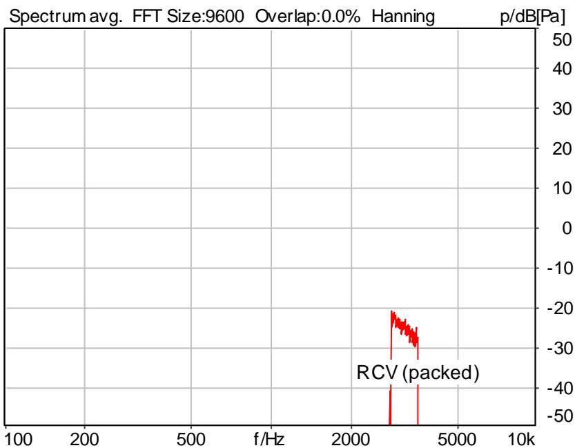
Distortion (Noise) RCV (packed): 42.39 dB (0.76%) Ok
