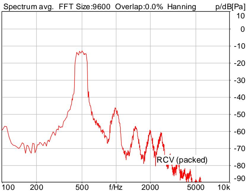
Distortion (Noise) RCV (packed): 30.86 dB (2.87%) Ok
