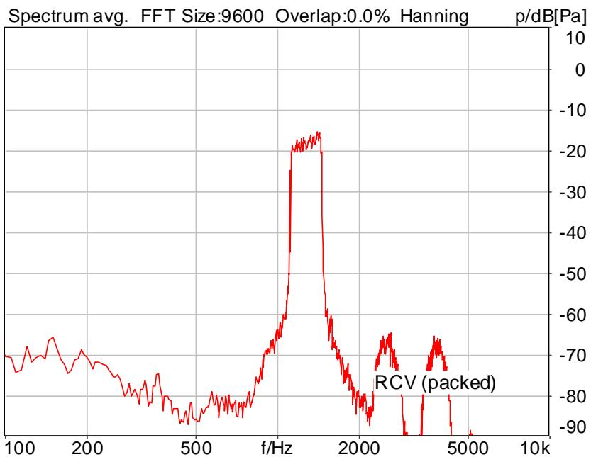
Distortion (Noise) RCV (packed): 33.17 dB (2.20%) Ok
