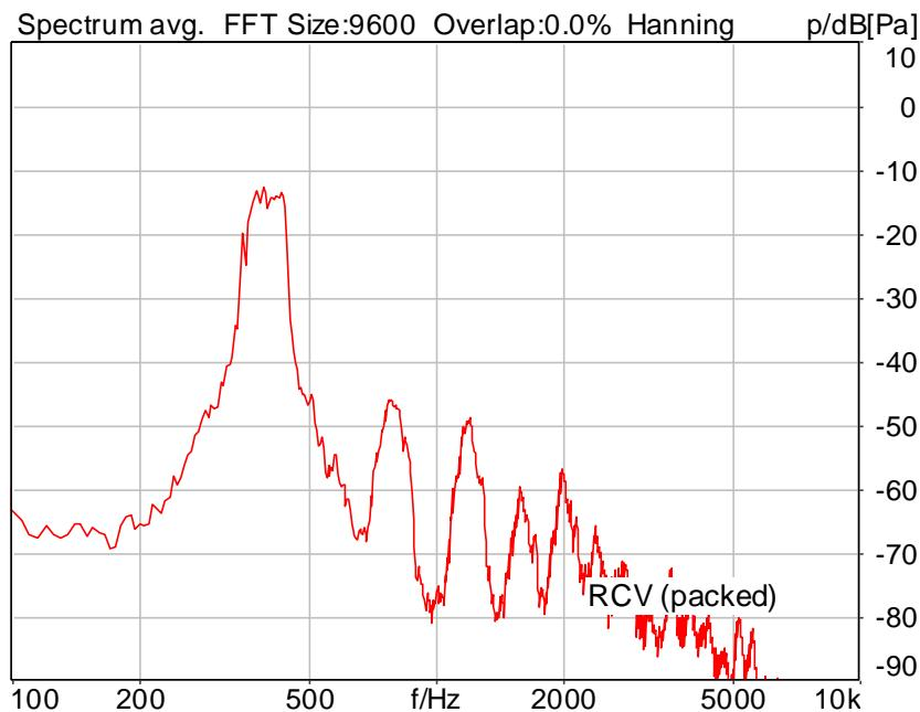
Distortion (Noise) RCV (packed): 29.13 dB (3.49%) Ok
