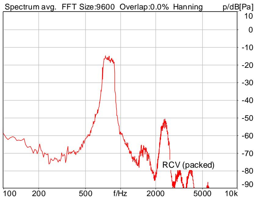
Distortion (Noise) RCV (packed): 29.77 dB (3.25%) Ok
