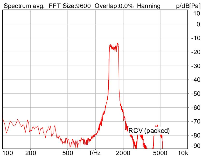
Distortion (Noise) RCV (packed): 40.30 dB (0.97%) Ok
