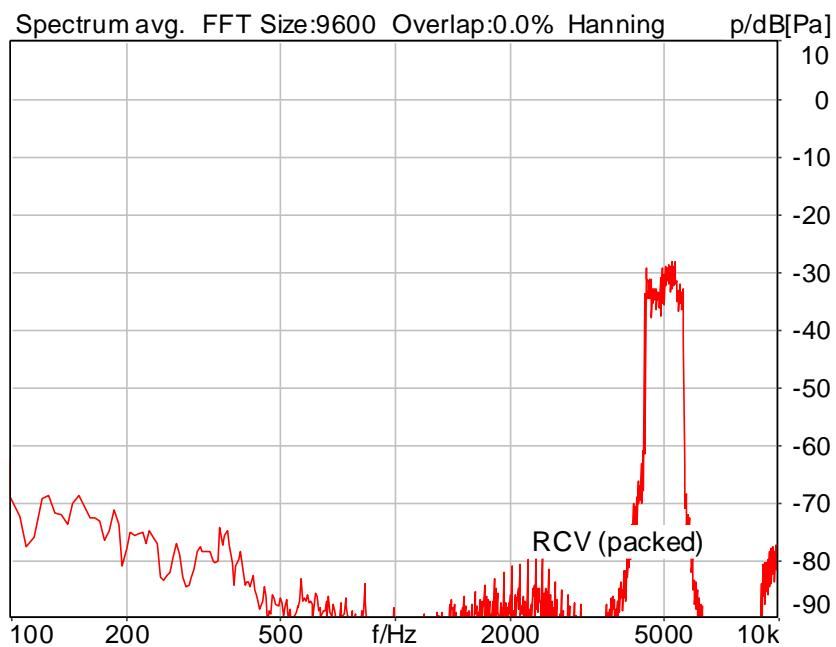
Distortion (Noise) RCV (packed): 39.56 dB (1.05%) Ok
