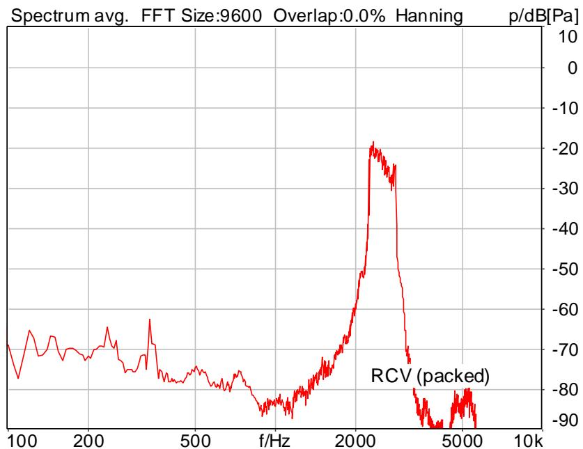
Distortion (Noise) RCV (packed): 28.97 dB (3.56%) Ok
