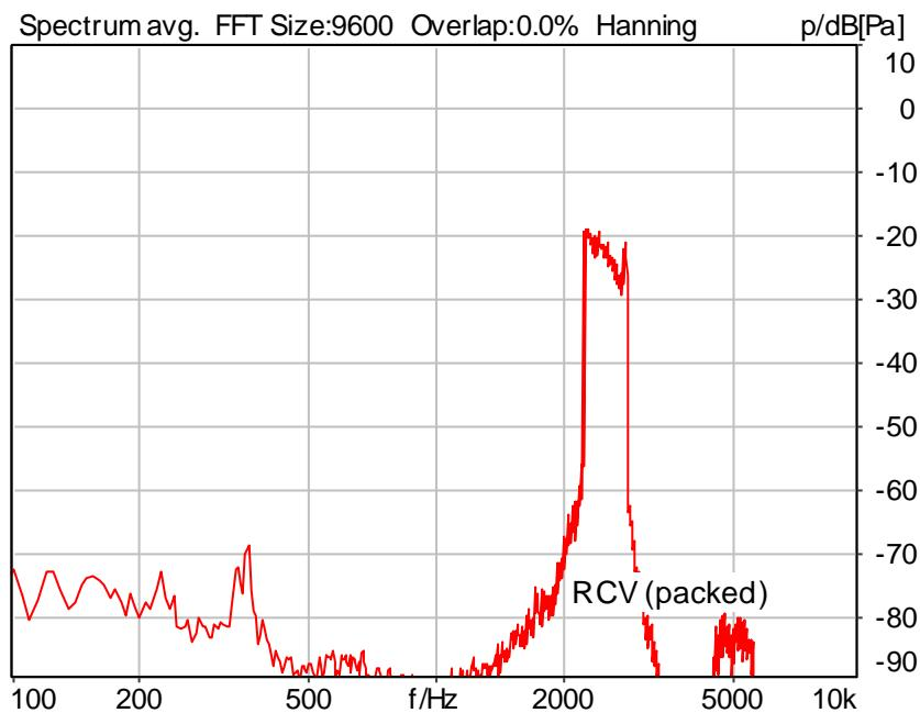
Distortion (Noise) RCV (packed): 43.46 dB (0.67%) Ok
