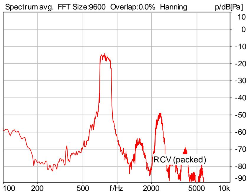
Distortion (Noise) RCV (packed): 30.64 dB (2.94%) Ok
