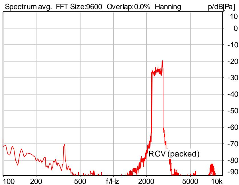
Distortion (Noise) RCV (packed): 42.36 dB (0.76%) Ok
