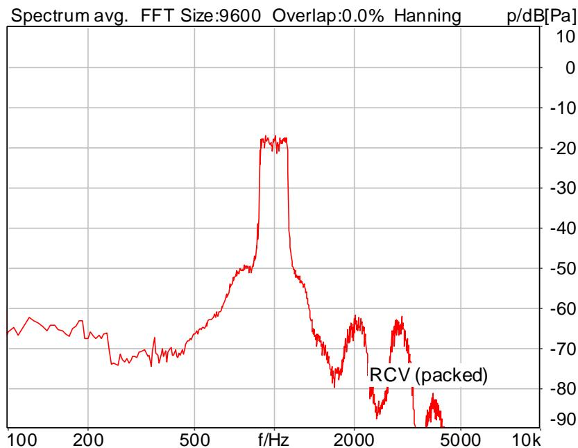
Distortion (Noise) RCV (packed): 30.60 dB (2.95%) Ok
