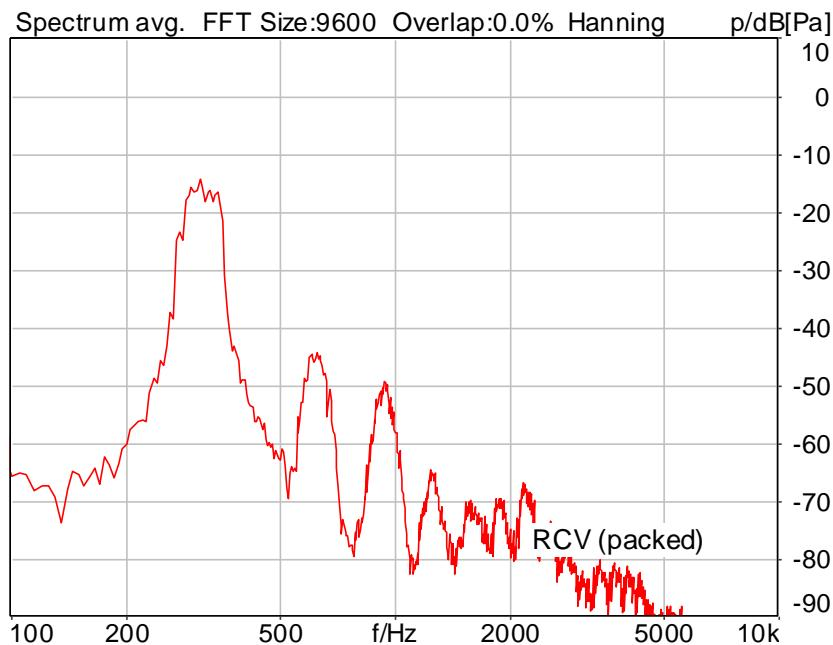
Distortion (Noise) RCV (packed): 28.16 dB (3.91%) Ok
