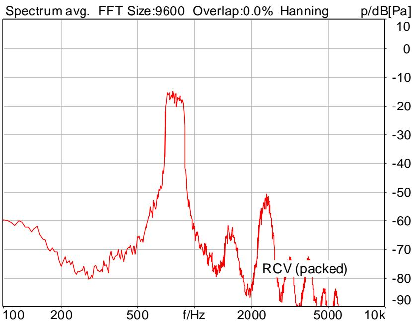
Distortion (Noise) RCV (packed): 31.69 dB (2.60%) Ok
