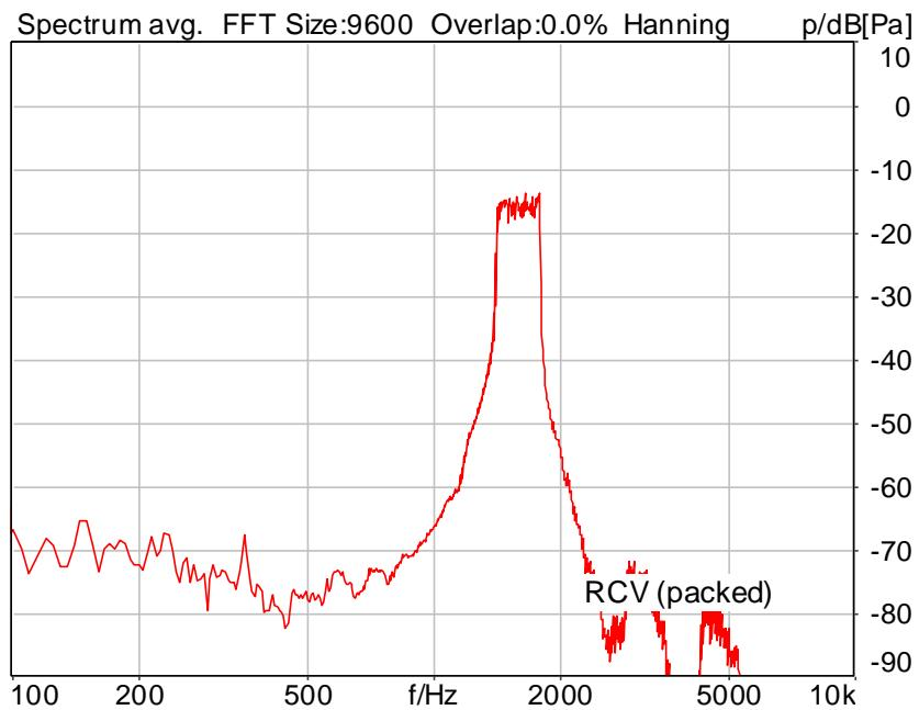
Distortion (Noise) RCV (packed): 29.71 dB (3.27%) Ok
