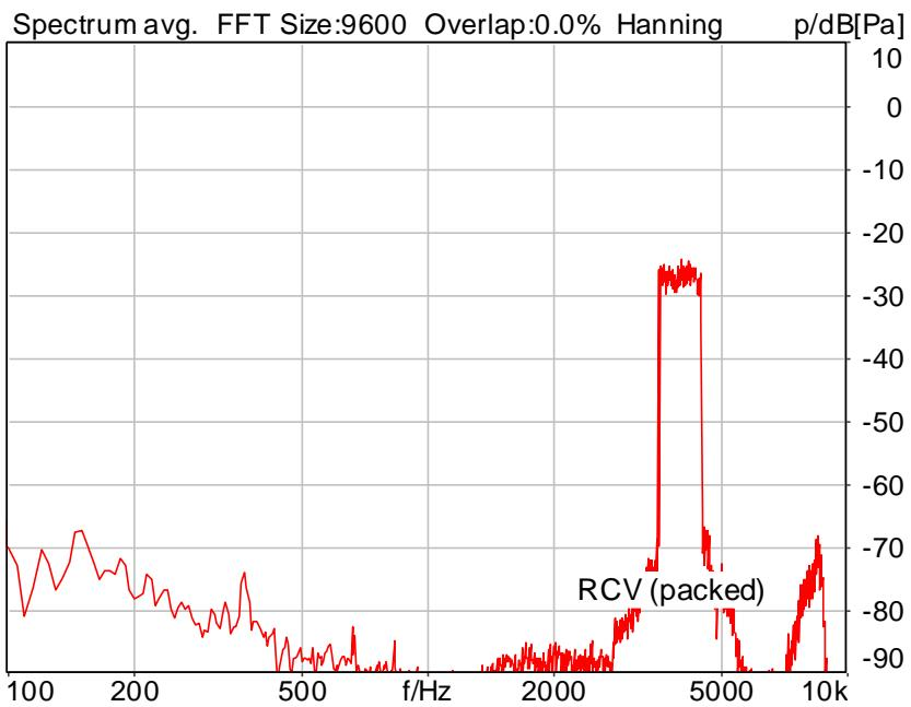
Distortion (Noise) RCV (packed): 44.16 dB (0.62%) Ok
