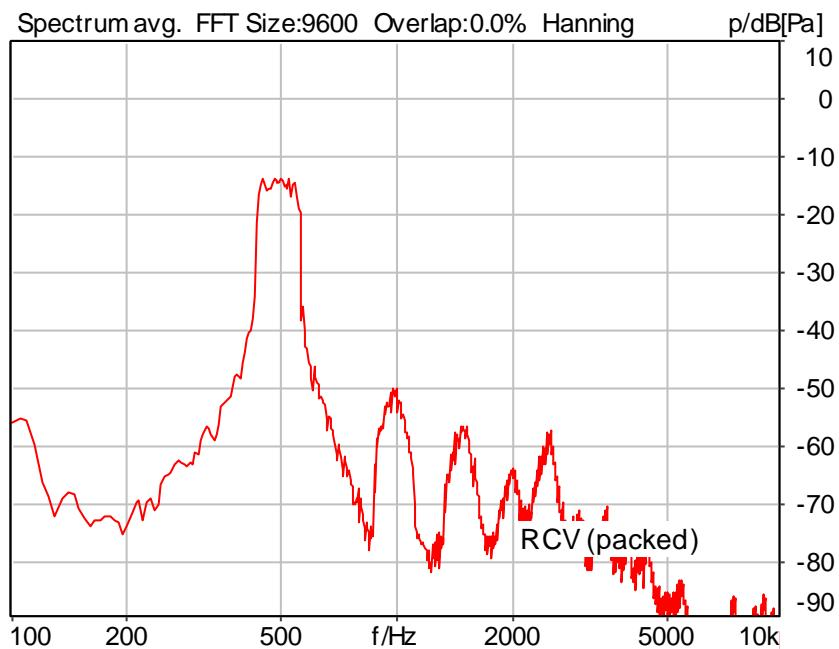
Distortion (Noise) RCV (packed): 32.26 dB (2.44%) Ok
