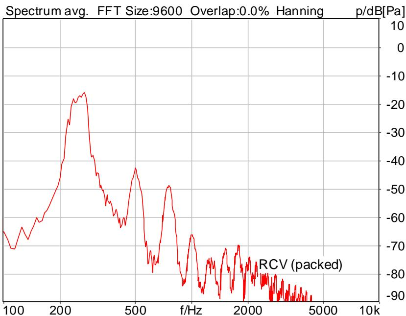
Distortion (Noise) RCV (packed): 27.22 dB (4.36%) Ok
