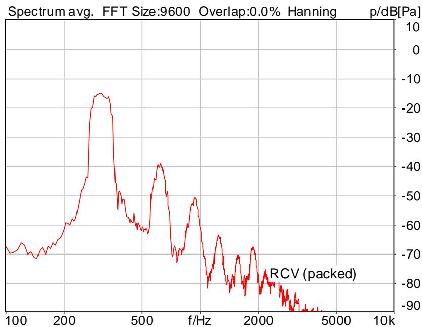
Distortion (Noise) RCV (packed): 25.33 dB (5.41%) Ok
