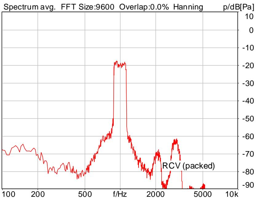
Distortion (Noise) RCV (packed): 37.22 dB (1.38%) Ok
