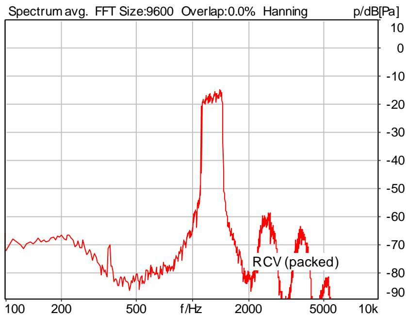
Distortion (Noise) RCV (packed): 31.59 dB (2.63%) Ok
