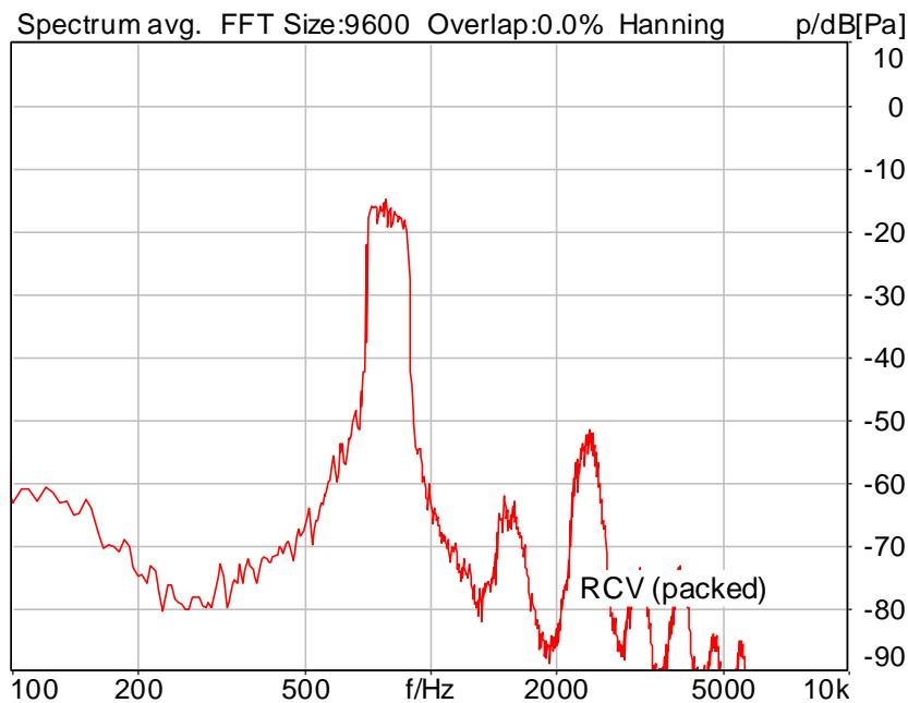
Distortion (Noise) RCV (packed): 32.02 dB (2.50%) Ok
