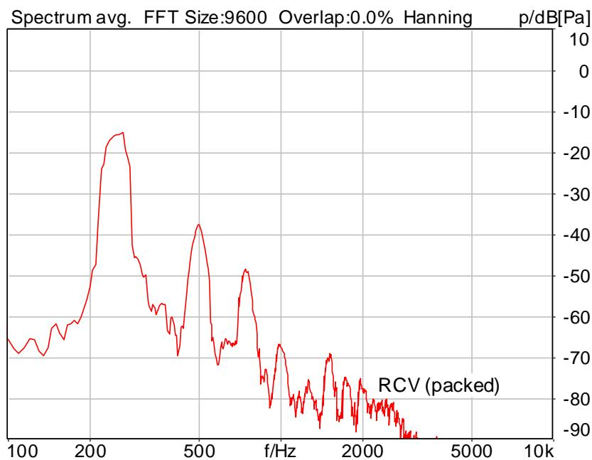
Distortion (Noise) RCV (packed): 24.73 dB (5.80%) Ok
