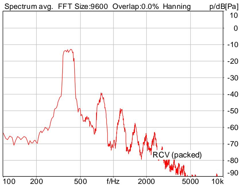
Distortion (Noise) RCV (packed): 26.71 dB (4.62%) Ok
