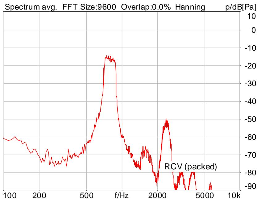
Distortion (Noise) RCV (packed): 30.58 dB (2.96%) Ok
