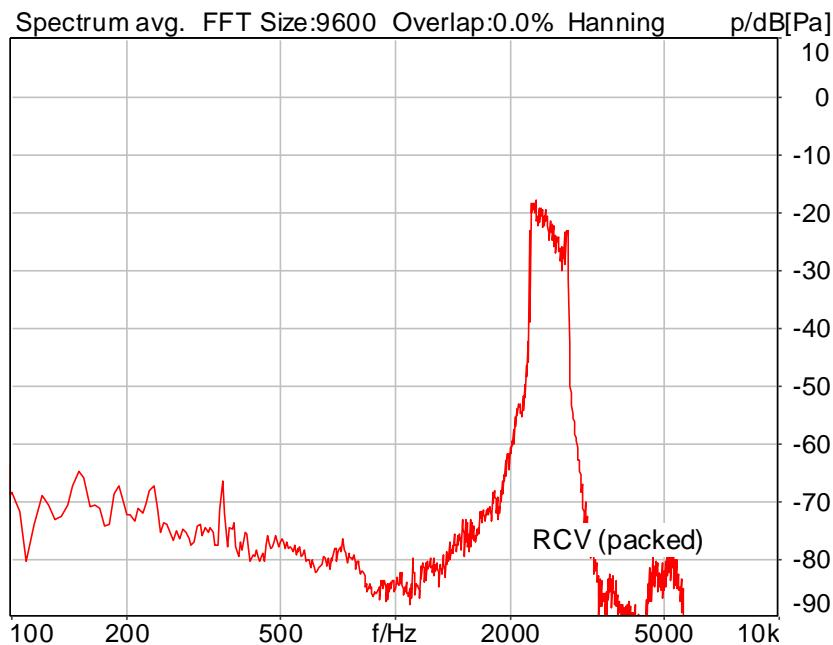
Distortion (Noise) RCV (packed): 32.82 dB (2.28%) Ok
