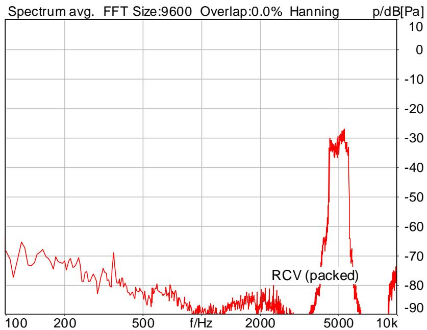
Distortion (Noise) RCV (packed): 34.04 dB (1.99%) Ok
