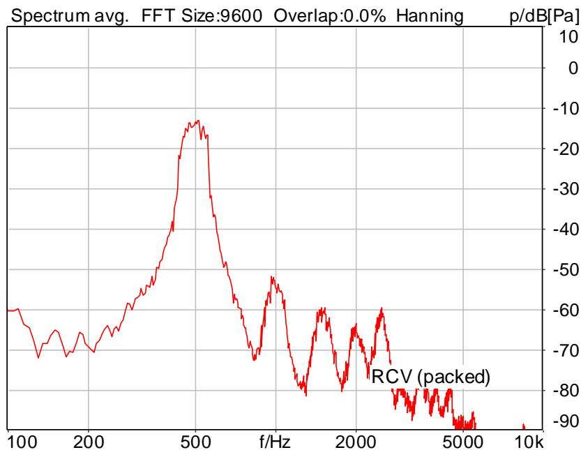
Distortion (Noise) RCV (packed): 30.80 dB (2.89%) Ok
