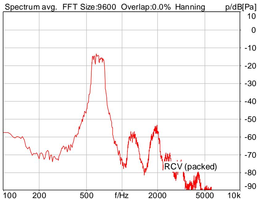
Distortion (Noise) RCV (packed): 30.63 dB (2.94%) Ok
