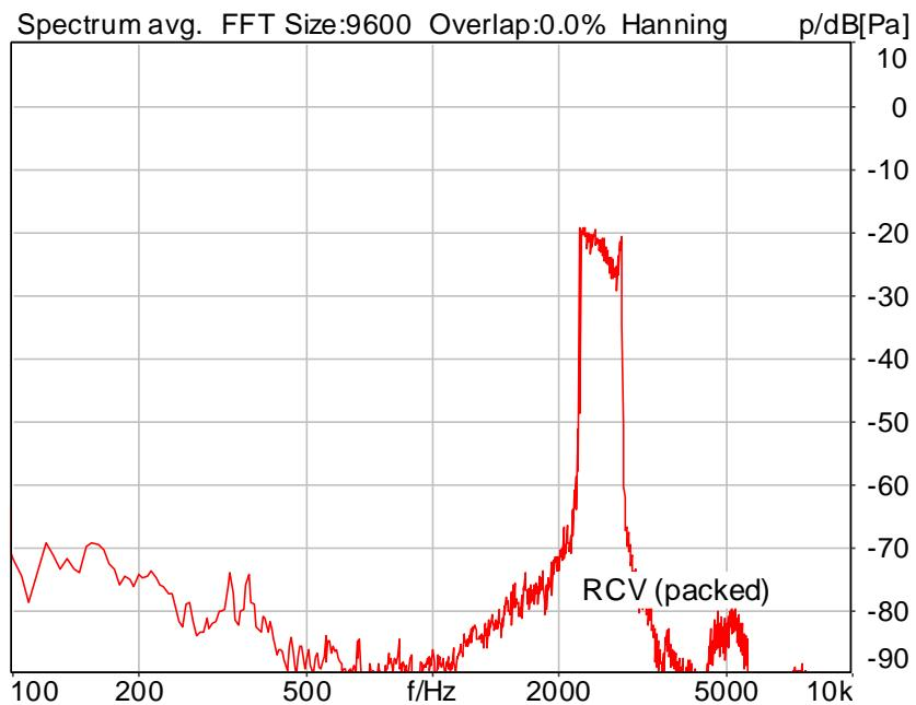
Distortion (Noise) RCV (packed): 44.69 dB (0.58%) Ok
