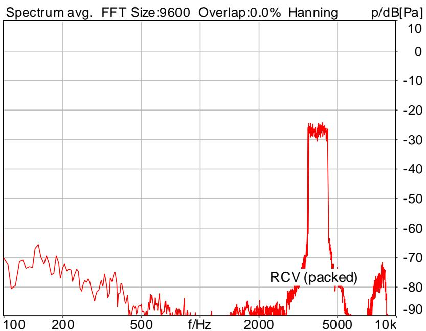
Distortion (Noise) RCV (packed): 42.51 dB (0.75%) Ok
