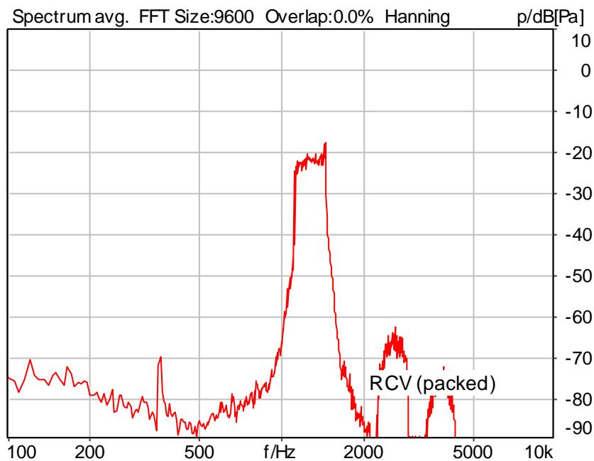
Distortion (Noise) RCV (packed): 22.38 dB (7.61%) Ok
