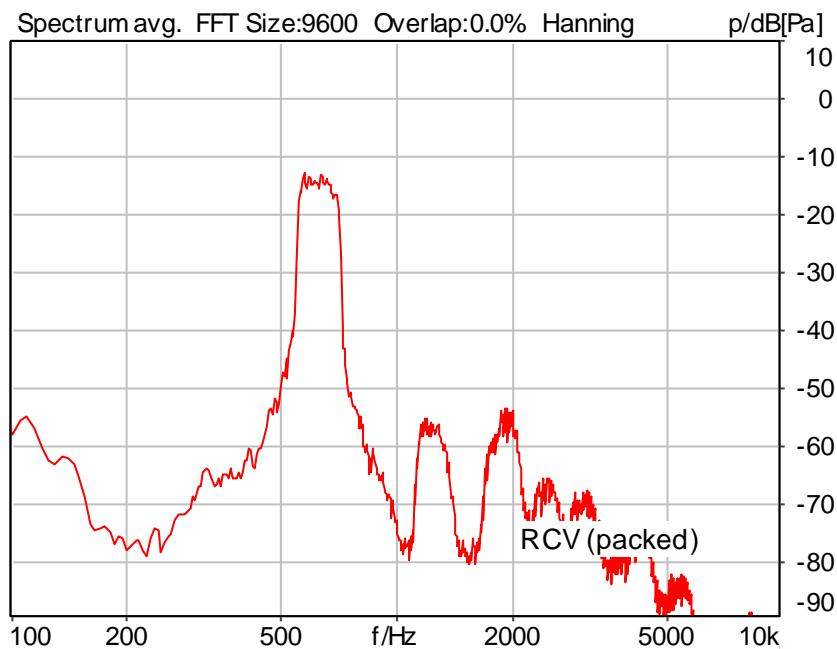
Distortion (Noise) RCV (packed): 33.72 dB (2.06%) Ok
