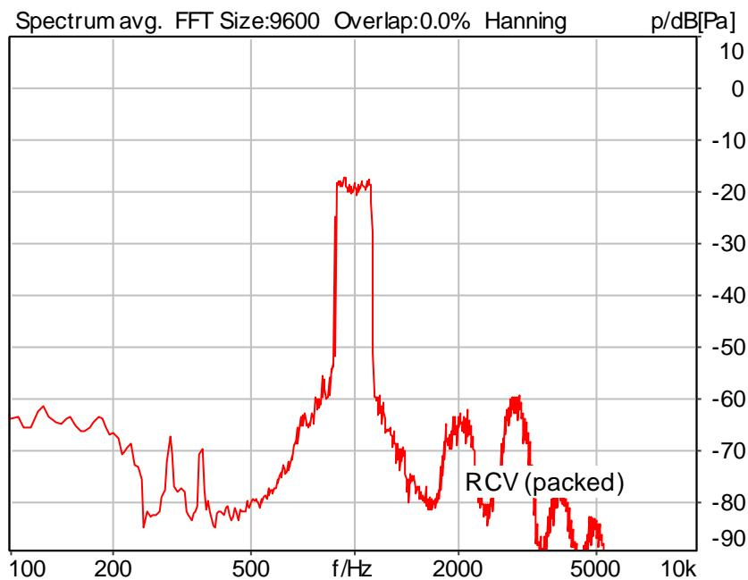
Distortion (Noise) RCV (packed): 36.39 dB (1.52%) Ok
