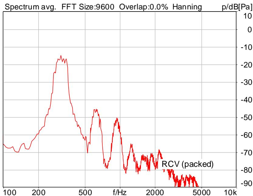
Distortion (Noise) RCV (packed): 28.36 dB (3.82%) Ok
