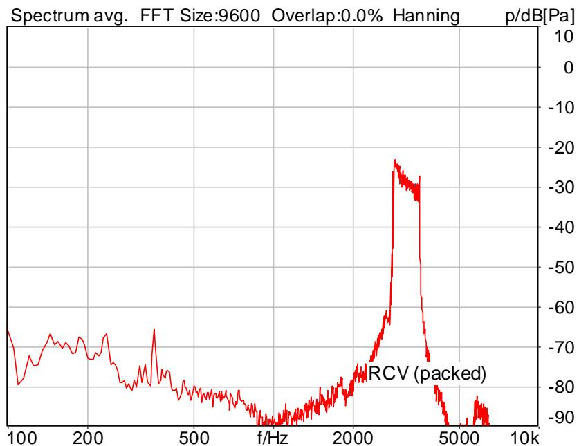
Distortion (Noise) RCV (packed): 34.43 dB (1.90%) Ok
