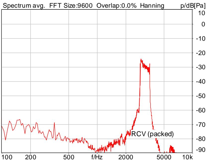
Distortion (Noise) RCV (packed): 31.48 dB (2.67%) Ok
