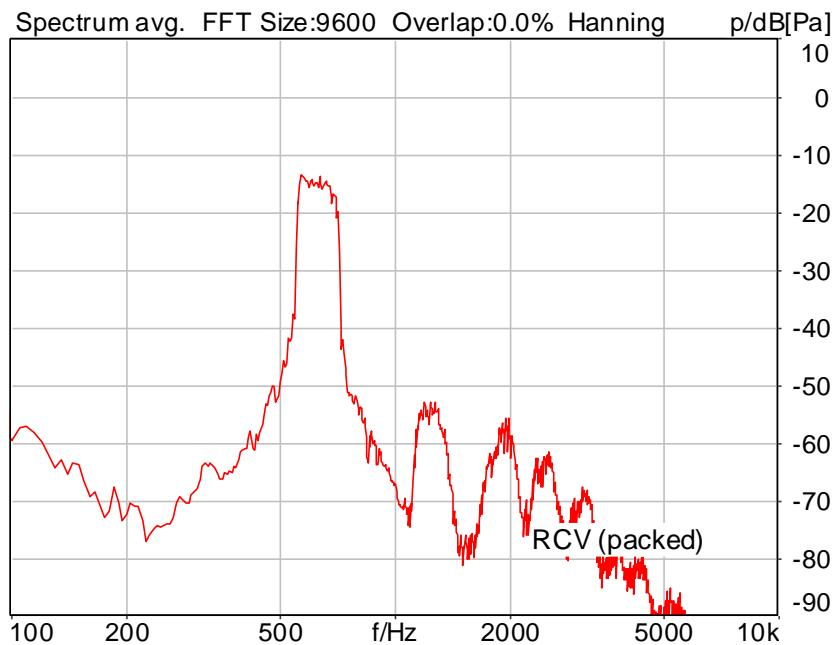
Distortion (Noise) RCV (packed): 32.76 dB (2.30%) Ok
