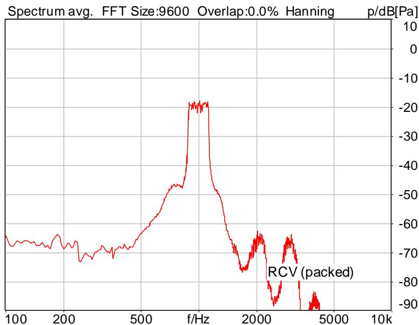
Distortion (Noise) RCV (packed): 26.55 dB (4.71%) Ok
