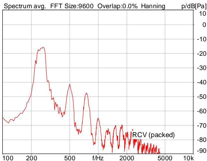
Distortion (Noise) RCV (packed): 27.05 dB (4.44%) Ok
