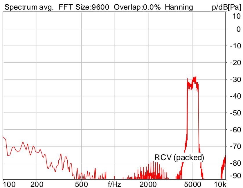
Distortion (Noise) RCV (packed): 40.72 dB (0.92%) Ok
