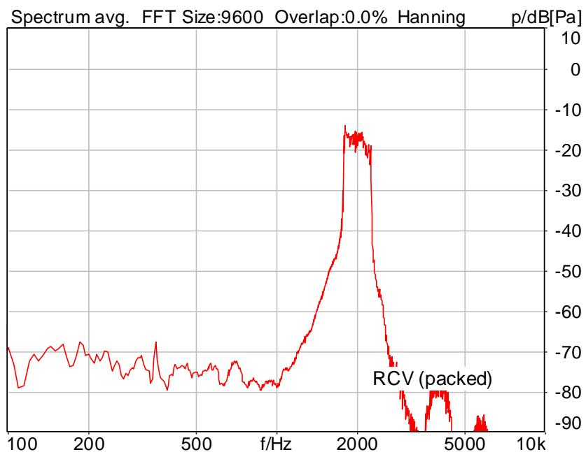
Distortion (Noise) RCV (packed): 29.58 dB (3.32%) Ok
