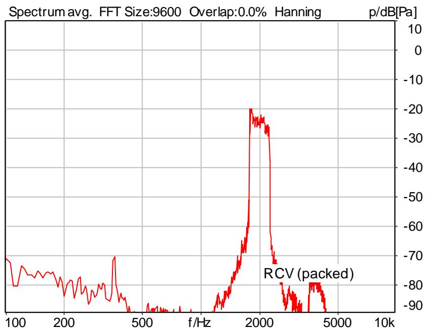
Distortion (Noise) RCV (packed): 42.62 dB (0.74%) Ok
