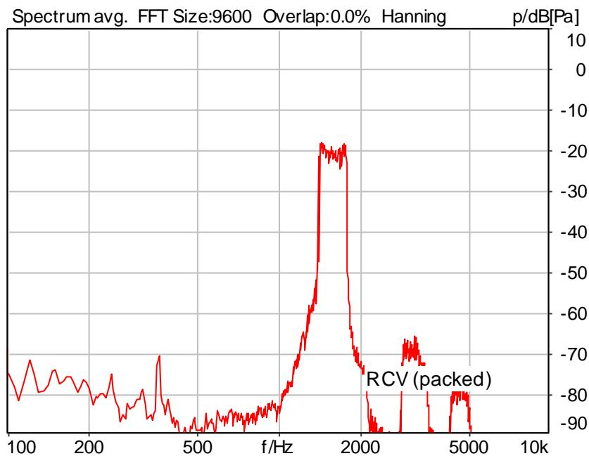
Distortion (Noise) RCV (packed): 39.90 dB (1.01%) Ok
