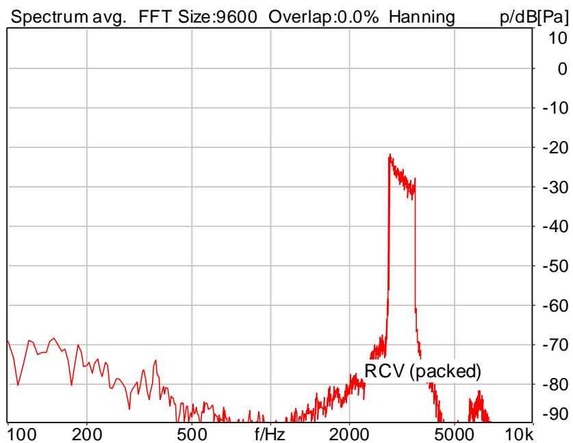
Distortion (Noise) RCV (packed): 41.98 dB (0.80%) Ok
