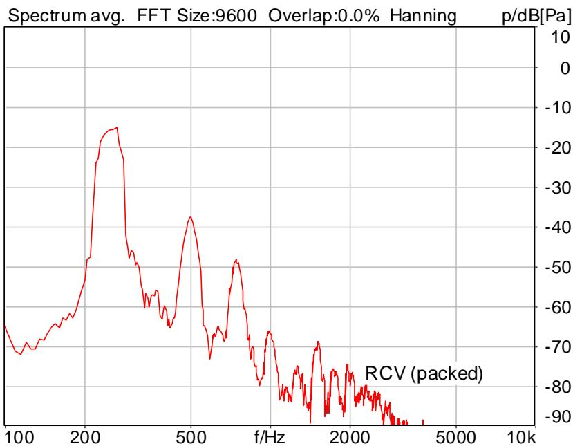
Distortion (Noise) RCV (packed): 24.75 dB (5.79%) Ok
