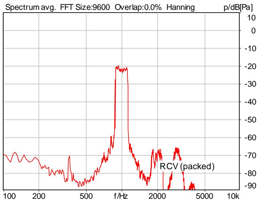
Distortion (Noise) RCV (packed): 38.89 dB (1.14%) Ok
