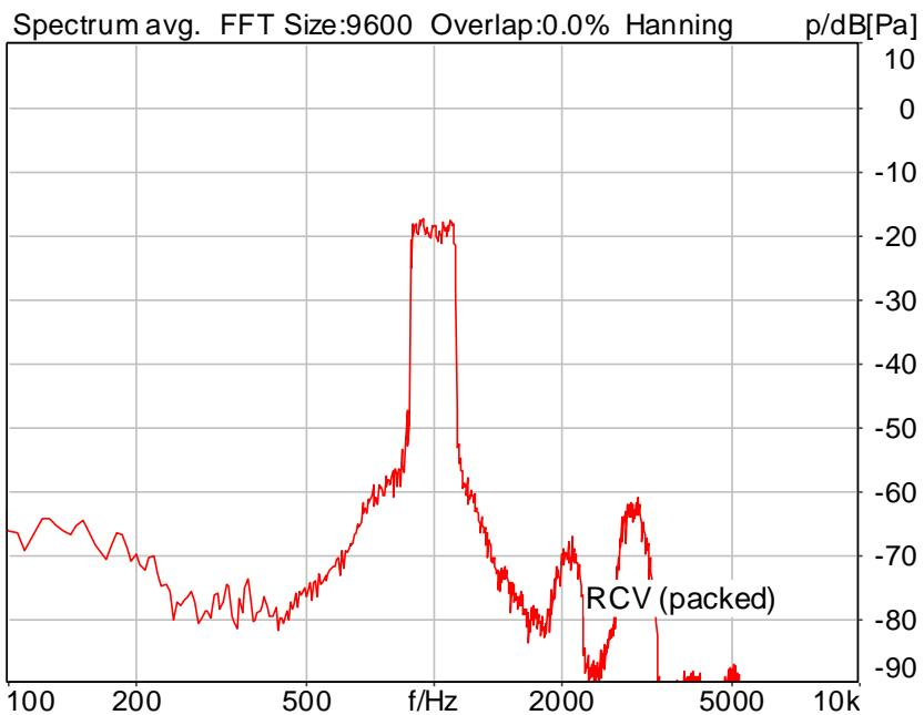
Distortion (Noise) RCV (packed): 36.72 dB (1.46%) Ok
