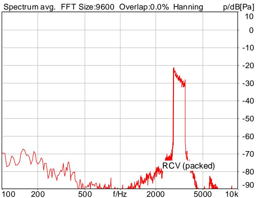
Distortion (Noise) RCV (packed): 43.20 dB (0.69%) Ok
