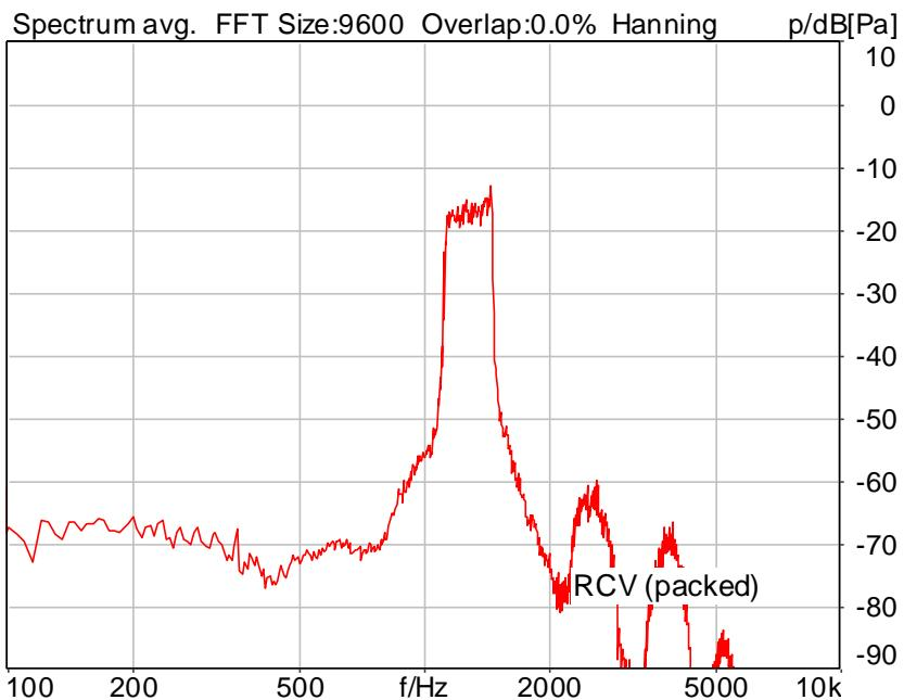
Distortion (Noise) RCV (packed): 25.52 dB (5.30%) Ok
