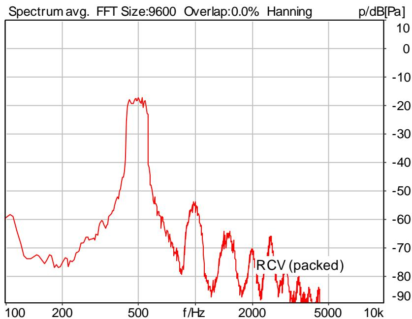
Distortion (Noise) RCV (packed): 33.96 dB (2.01%) Ok
