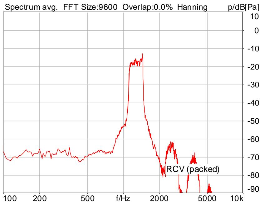
Distortion (Noise) RCV (packed): 22.90 dB (7.16%) Ok
