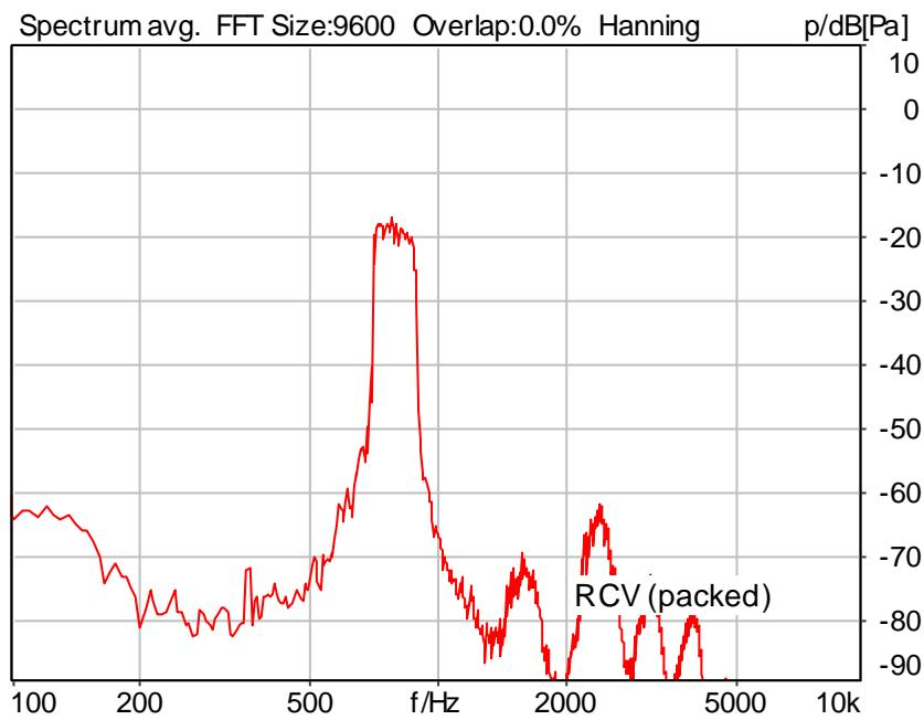
Distortion (Noise) RCV (packed): 38.08 dB (1.25%) Ok
