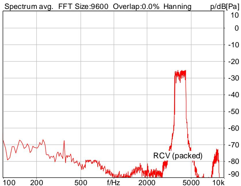
Distortion (Noise) RCV (packed): 34.66 dB (1.85%) Ok
