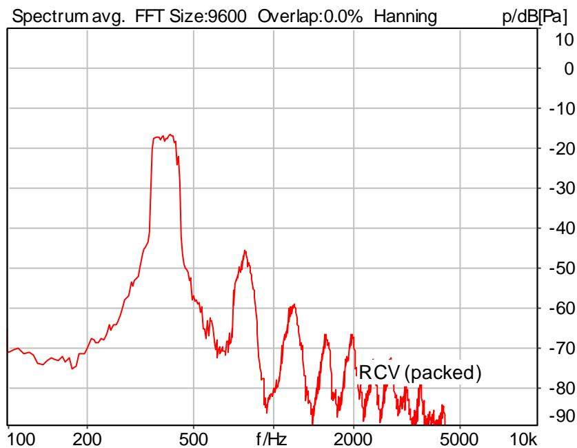
Distortion (Noise) RCV (packed): 30.04 dB (3.15%) Ok
