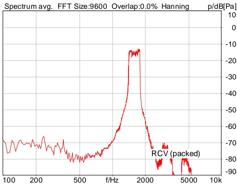
Distortion (Noise) RCV (packed): 32.99 dB (2.24%) Ok
