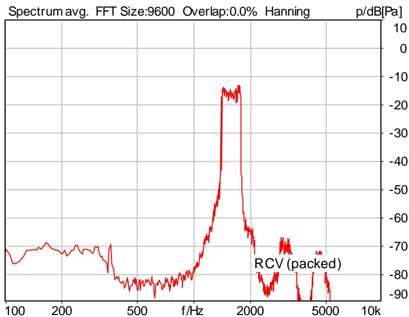
Distortion (Noise) RCV (packed): 41.18 dB (0.87%) Ok
