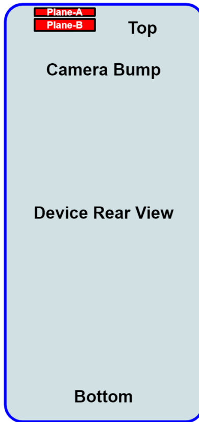
Figure 1-1 Placement of the L-shaped mmWave modules, called Plane-A sub-module and Plane-B sub-module, positioned at the top and back side of the device, respectively.
