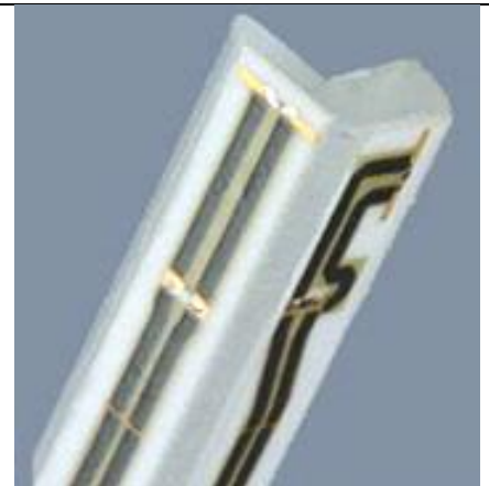
Fig 5.2 Photo of E-field Probe
