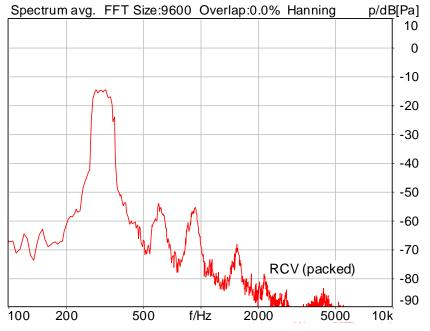
Distortion (Noise) RCV (packed): 37.02 dB (1.41%) Ok
