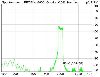
Distortion (Noise) RCV (packed): 43.14 dB (0.70%) Ok
