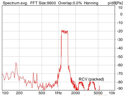
Distortion (Noise) RCV (packed): 32.92 dB (2.26%) Ok
