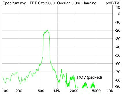
Distortion (Noise) RCV (packed): 39.39 dB (1.07%) Ok
