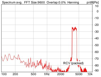
Distortion (Noise) RCV (packed): 44.72 dB (0.58%) Ok
