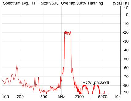
Distortion (Noise) RCV (packed): 32.80 dB (2.29%) Ok
