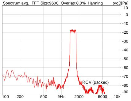
Distortion (Noise) RCV (packed): 45.26 dB (0.55%) Ok
