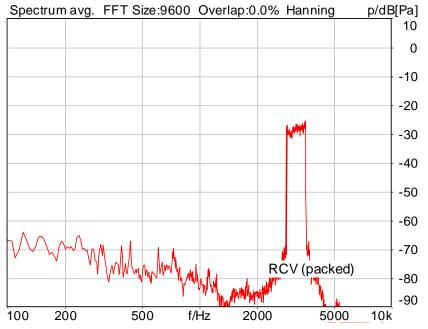
Distortion (Noise) RCV (packed): 42.67 dB (0.74%) Ok
