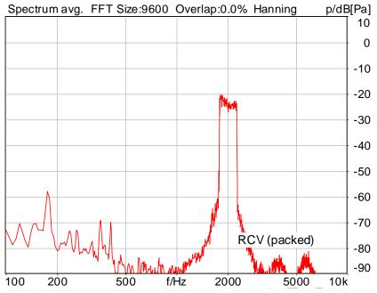
Distortion (Noise) RCV (packed): 42.90 dB (0.72%) Ok
