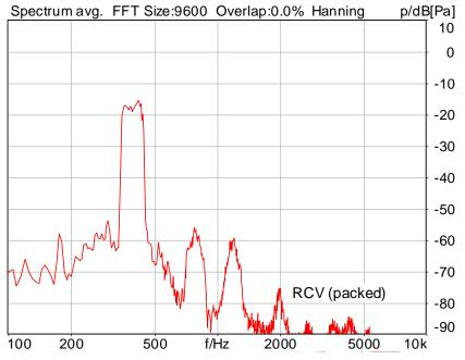
Distortion (Noise) RCV (packed): 37.77 dB (1.29%) Ok
