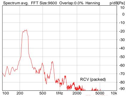
Distortion (Noise) RCV (packed): 35.23 dB (1.73%) Ok
