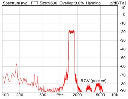
Distortion (Noise) RCV (packed): 48.81 dB (0.36%) Ok
