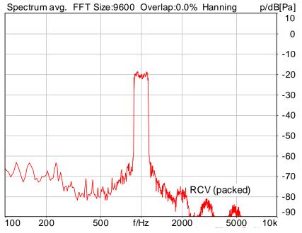
Distortion (Noise) RCV (packed): 44.47 dB (0.60%) Ok
