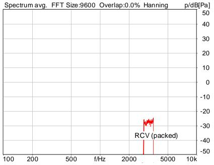
Distortion (Noise) RCV (packed): 32.58 dB (2.35%) Ok
