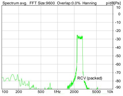
Distortion (Noise) RCV (packed): 44.10 dB (0.62%) Ok
