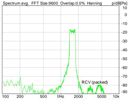
Distortion (Noise) RCV (packed): 42.17 dB (0.78%) Ok
