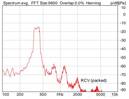
Distortion (Noise) RCV (packed): 38.15 dB (1.24%) Ok
