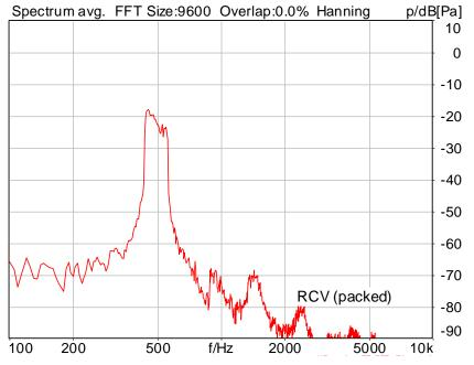
Distortion (Noise) RCV (packed): 37.62 dB (1.31%) Ok
