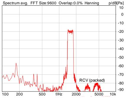
Distortion (Noise) RCV (packed): 48.76 dB (0.36%) Ok
