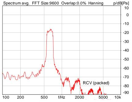
Distortion (Noise) RCV (packed): 39.48 dB (1.06%) Ok
