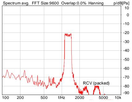
Distortion (Noise) RCV (packed): 32.34 dB (2.42%) Ok
