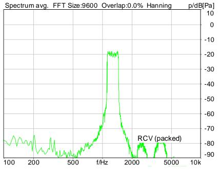
Distortion (Noise) RCV (packed): 31.77 dB (2.58%) Ok
