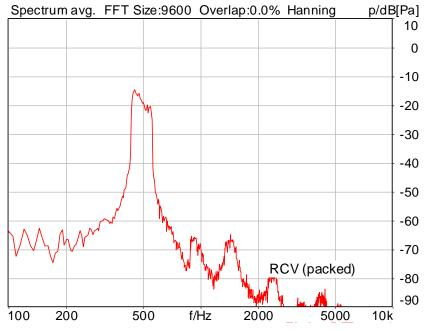
Distortion (Noise) RCV (packed): 38.10 dB (1.25%) Ok
