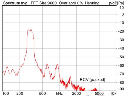
Distortion (Noise) RCV (packed): 36.48 dB (1.50%) Ok
