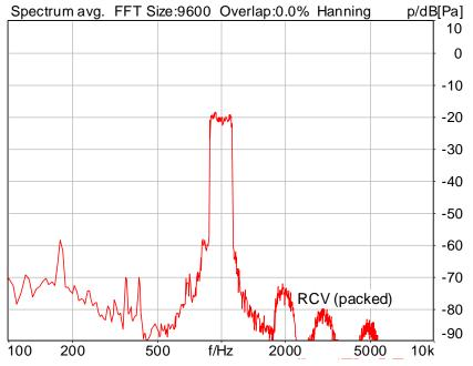
Distortion (Noise) RCV (packed): 43.62 dB (0.66%) Ok
