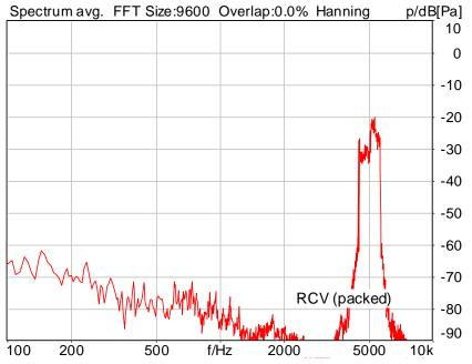
Distortion (Noise) RCV (packed): 40.80 dB (0.91%) Ok
