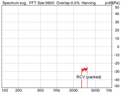
Distortion (Noise) RCV (packed): 32.63 dB (2.34%) Ok
