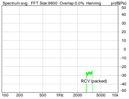
Distortion (Noise) RCV (packed): 42.89 dB (0.72%) Ok
