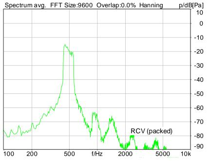
Distortion (Noise) RCV (packed): 37.88 dB (1.28%) Ok
