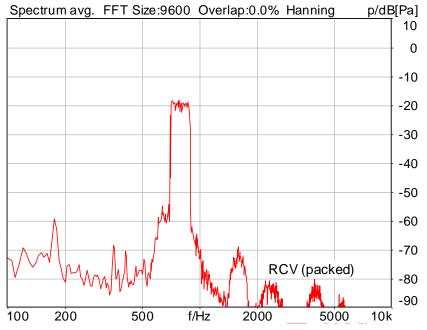
Distortion (Noise) RCV (packed): 42.61 dB (0.74%) Ok
