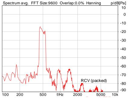
Distortion (Noise) RCV (packed): 40.89 dB (0.90%) Ok
