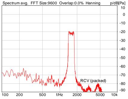
Distortion (Noise) RCV (packed): 44.34 dB (0.61%) Ok
