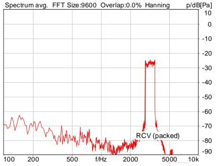
Distortion (Noise) RCV (packed): 43.06 dB (0.70%) Ok
