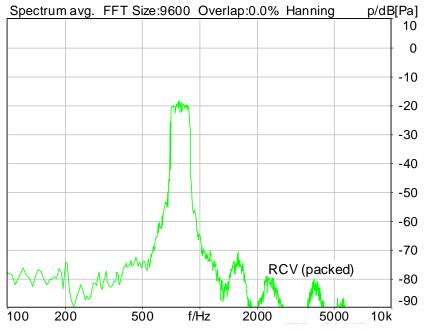
Distortion (Noise) RCV (packed): 39.32 dB (1.08%) Ok
