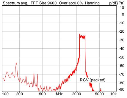
Distortion (Noise) RCV (packed): 31.41 dB (2.69%) Ok
