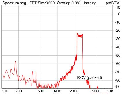
Distortion (Noise) RCV (packed): 31.38 dB (2.70%) Ok
