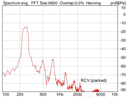
Distortion (Noise) RCV (packed): 35.30 dB (1.72%) Ok
