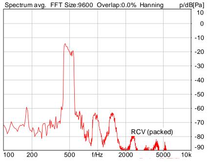
Distortion (Noise) RCV (packed): 40.92 dB (0.90%) Ok
