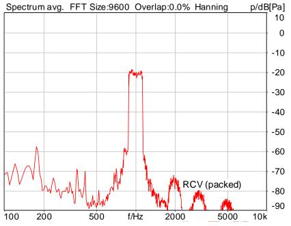
Distortion (Noise) RCV (packed): 43.56 dB (0.66%) Ok
