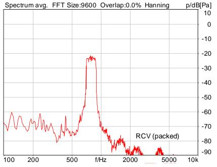
Distortion (Noise) RCV (packed): 38.64 dB (1.17%) Ok
