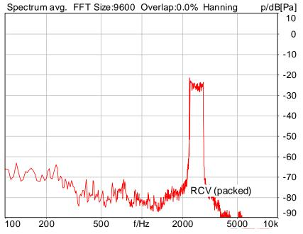
Distortion (Noise) RCV (packed): 43.70 dB (0.65%) Ok
