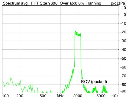
Distortion (Noise) RCV (packed): 43.42 dB (0.67%) Ok
