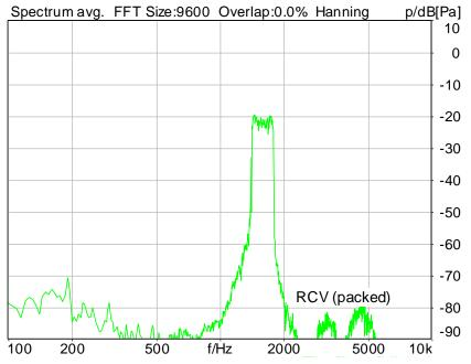
Distortion (Noise) RCV (packed): 42.04 dB (0.79%) Ok
