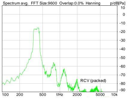
Distortion (Noise) RCV (packed): 37.87 dB (1.28%) Ok
