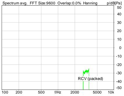
Distortion (Noise) RCV (packed): 44.52 dB (0.59%) Ok
