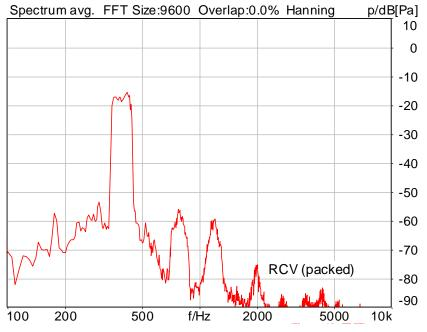
Distortion (Noise) RCV (packed): 37.72 dB (1.30%) Ok
