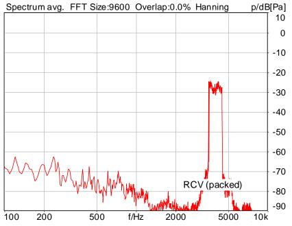
Distortion (Noise) RCV (packed): 43.84 dB (0.64%) Ok
