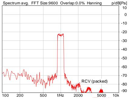
Distortion (Noise) RCV (packed): 43.87 dB (0.64%) Ok
