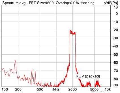
Distortion (Noise) RCV (packed): 42.86 dB (0.72%) Ok
