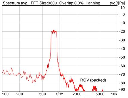
Distortion (Noise) RCV (packed): 39.07 dB (1.11%) Ok
