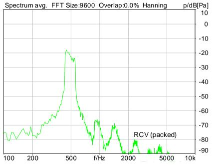
Distortion (Noise) RCV (packed): 37.76 dB (1.29%) Ok
