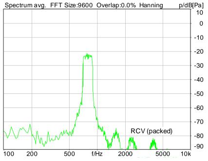
Distortion (Noise) RCV (packed): 39.16 dB (1.10%) Ok
