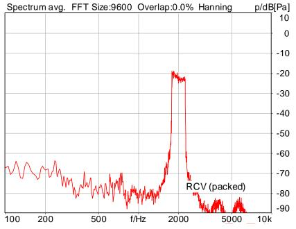
Distortion (Noise) RCV (packed): 41.57 dB (0.83%) Ok
