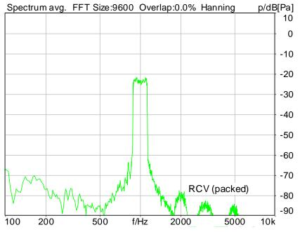
Distortion (Noise) RCV (packed): 44.01 dB (0.63%) Ok
