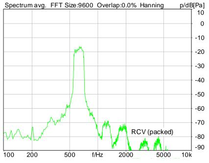
Distortion (Noise) RCV (packed): 39.61 dB (1.05%) Ok
