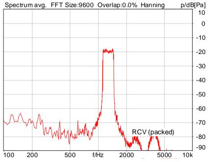
Distortion (Noise) RCV (packed): 29.57 dB (3.32%) Ok
