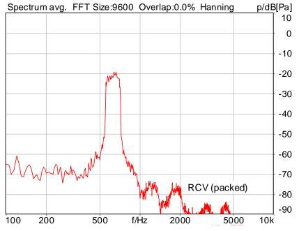
Distortion (Noise) RCV (packed): 39.17 dB (1.10%) Ok
