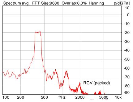
Distortion (Noise) RCV (packed): 38.05 dB (1.25%) Ok
