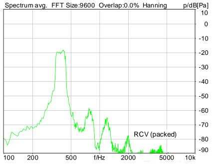
Distortion (Noise) RCV (packed): 37.85 dB (1.28%) Ok
