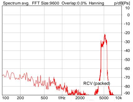
Distortion (Noise) RCV (packed): 41.42 dB (0.85%) Ok
