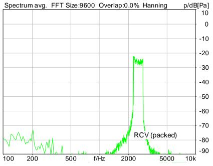
Distortion (Noise) RCV (packed): 43.60 dB (0.66%) Ok
