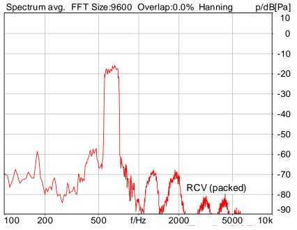
Distortion (Noise) RCV (packed): 42.91 dB (0.72%) Ok
