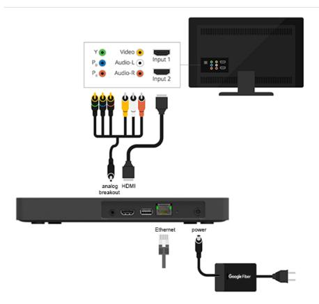
When the TV Box is properly connected and powered on, the LED on the front displays solid blue.
