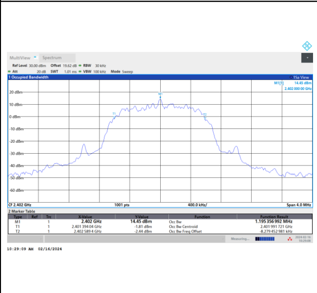
99% Occupied Bandwidth Plot on Channel 78
