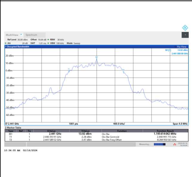
99% Occupied Plot Bandwidth on Channel 39
