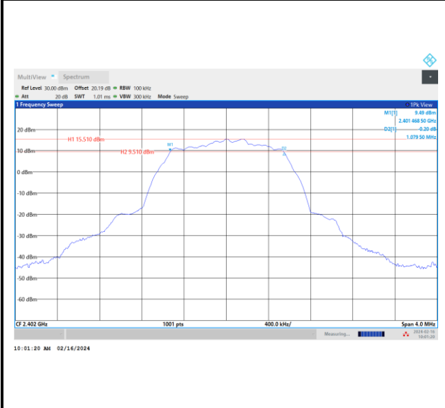
6 dB Bandwidth Plot on Channel 78
