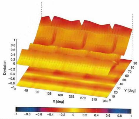
Probe isotropy for  $E_{tot}$ : probe rotated  $\phi=0^\circ$  to 360°, tilted from field propagation direction  $\vec{k}$  Parallel to the field propagation ( $\psi=0^\circ-90^\circ$ ) at 30 GHz: deviation within  $\pm 0.31$  dB Parallel to the field propagation ( $\psi=0^\circ-90^\circ$ ) at 60 GHz: deviation within  $\pm 0.40$  dB
