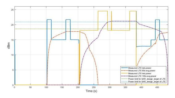
Figure 7.6-3 Conducted TxPower in SAR Window Change test
