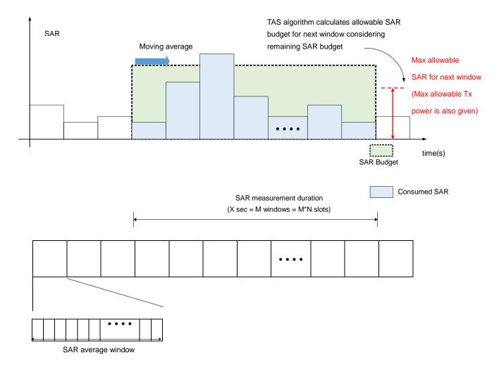
Average SAR value in a slot can be calculated from average Tx power in the slot (Assume that SAR vs Tx power relation is obtained from real measurement)
