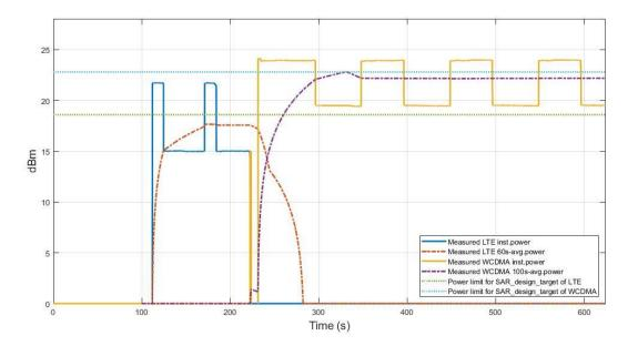
Figure 7.5-1 Conducted Tx power for Wireless technology Handover
