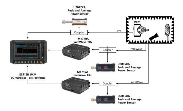
Figure 8.1-1 Test set-up for mmWave
