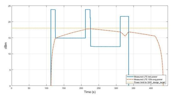
Figure 7.10-1 Conducted transmitted power of LTE Band 5 in UL CA
