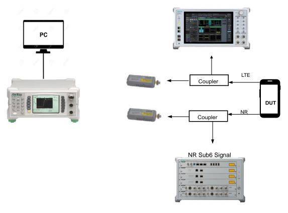
Figure 7.1-1 Test set-up for legacy and sub 6GHz
