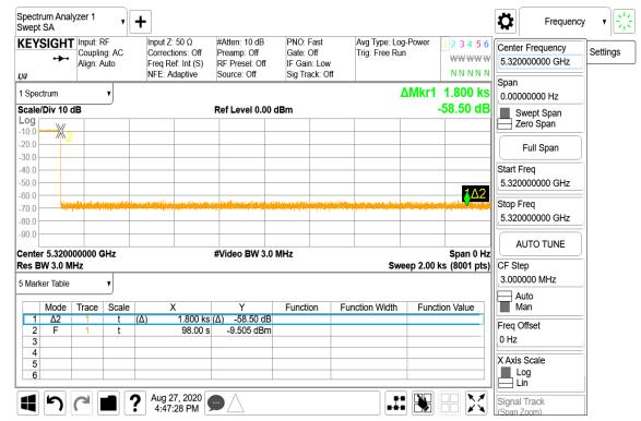
**Verdict:** To verify whether channel is unavailable to be operated in 30 minutes. 1.8ks = 1800s = 1800 s/min /60 = 30 minute
