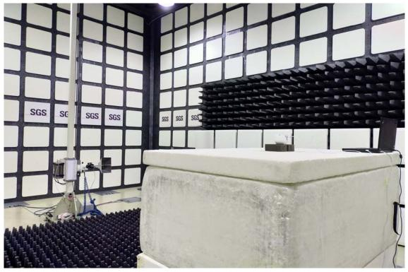
Radiated Emission Set up Photos (Front View)
