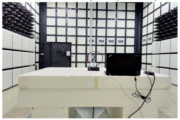
Radiated Emission Set up Photos (Below 1GHz)
