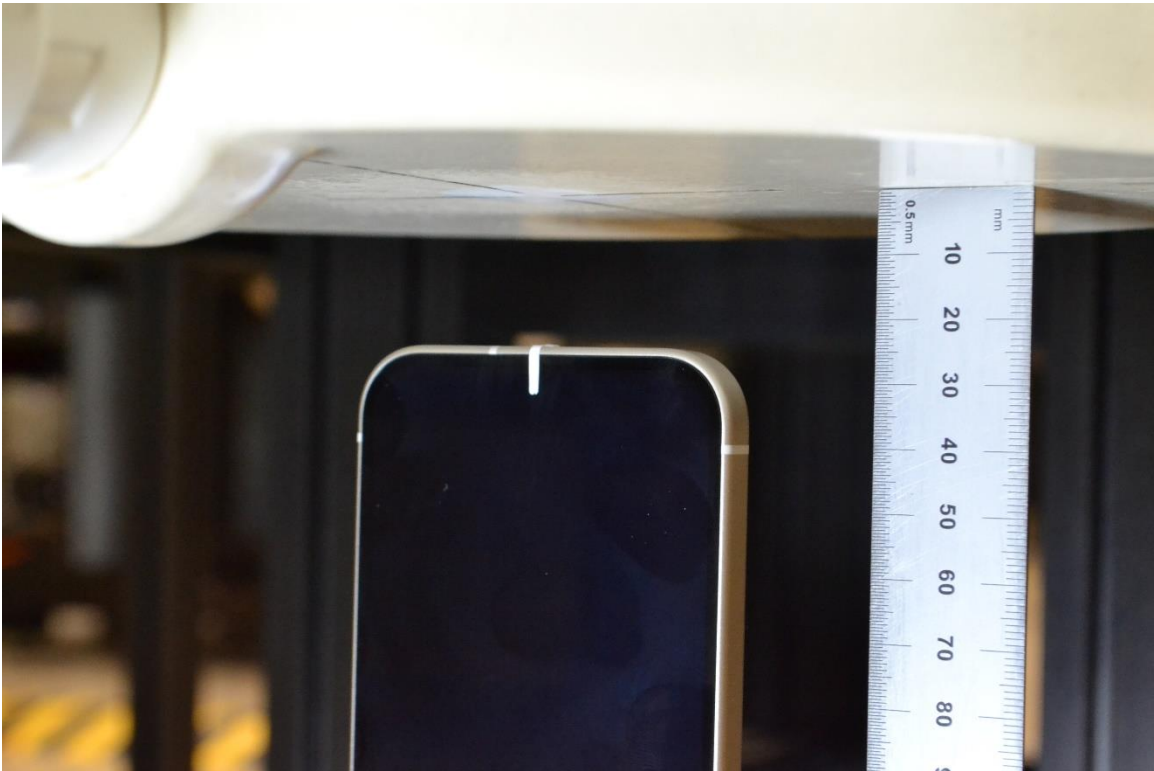
Photograph 18: Hotspot, Edge Bottom, 25 mm
