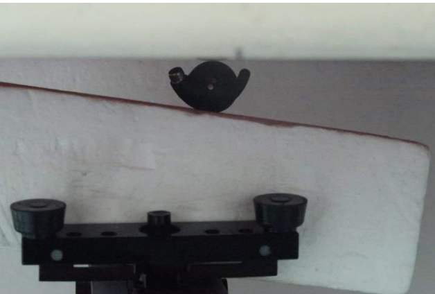
Antenna Side, Test Separation 0 mm
