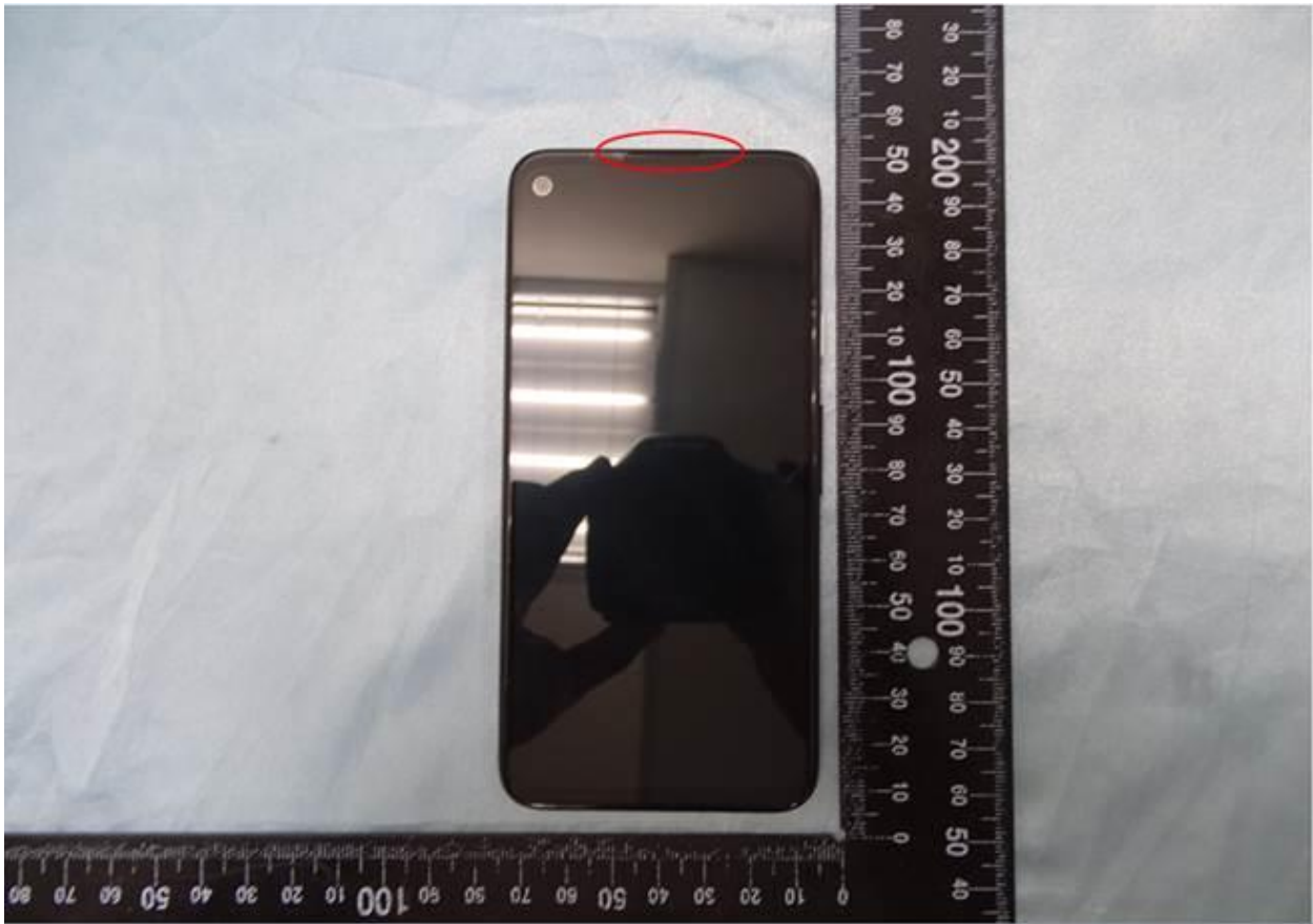
The center of the acoustic output of EUT is positioned on the reference line of Test Arch phantom
