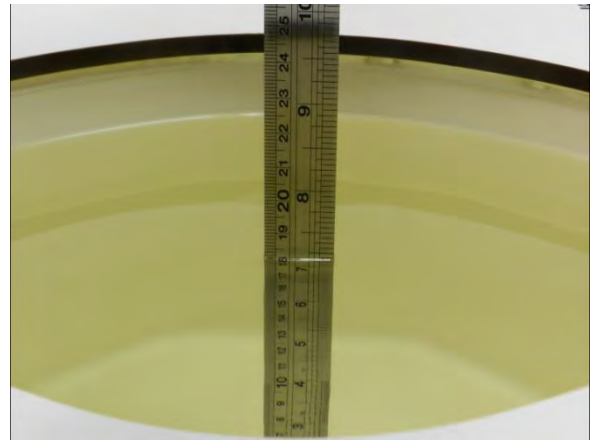
Fig 10.2 Photo of Liquid Height for Body SAR
