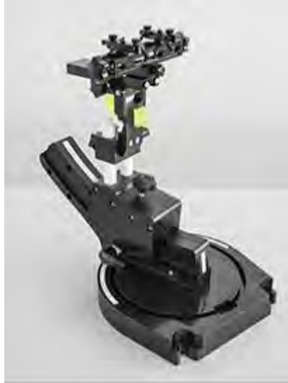
Mounting Device for Hand-Held Transmitters
