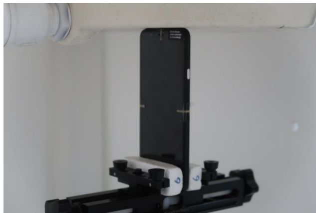
Top Side, Test Separation 0 mm
