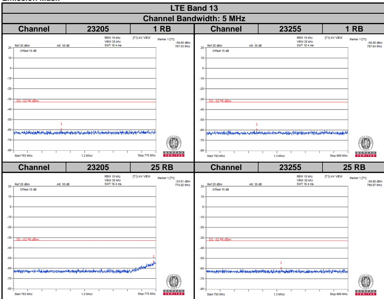
For the 763 - 775 MHz and 793 - 805 MHz band, the FCC limit is  $65 + 10\log(P[\text{watt}])$  in a 6.25 kHz bandwidth. Since it was not possible to set the resolution bandwidth to 6.25 kHz with the available equipment, a bandwidth of 10 kHz was used instead to show compliance. By using a 10 kHz bandwidth on the spectrum analyzer.
