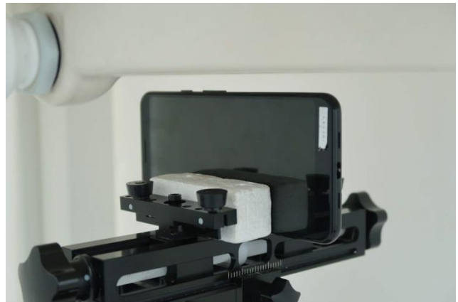
Right Side, Test Separation 10 mm
