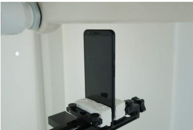
Top Side, Test Separation 10 mm
