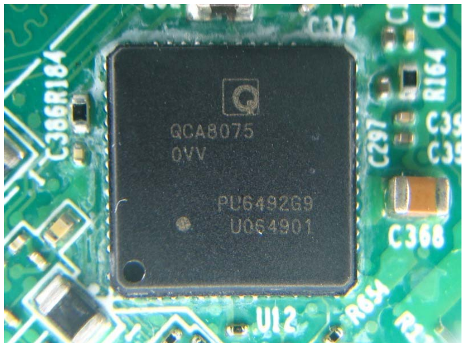
Source: PHY Second source Model Name: QCA8075
