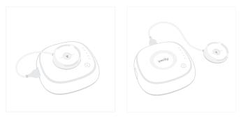
Plug the Study Watch's charging dock into one of the USB ports, either on the side of the Hub or at the back. You can put the dock either on top of the Study Hub or to the side.
