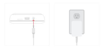
Plug the power cord into the round port on the back of the Study Hub.
