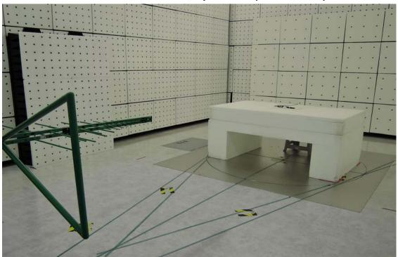
Radiated Emission Set up Photos (Above 1GHz)
