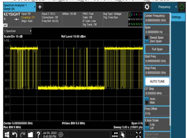
Det LeI_802.11ax_20MHz_CF 6695MHz_6695MHzMHz_-72.2dBm
