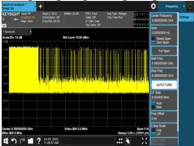
Det Le1_802.11ax_160MHz_CF 6665MHz_6590MHz_-69.33dBm
