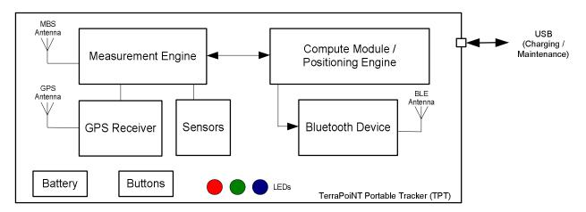
The TPT receiver system comprises of a measurement engine (ME) block, a compute module block, gps receiver and different sensors. The measurement engine block performs the acquisition and tracking of MBS beacon signals. The compute module receives the ME data and computes the ranges and trilateration to produce location fixes at 10Hz rate. The receiver is designed to interact and deliver location fixes to a host platform (Smart Phone) via Bluetooth.
