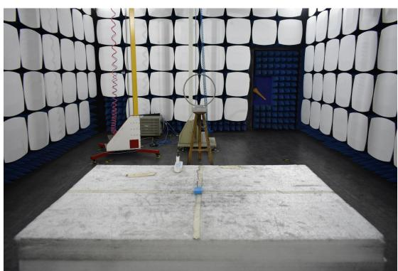
3. Radiated emission (9KHz-30MHz)
