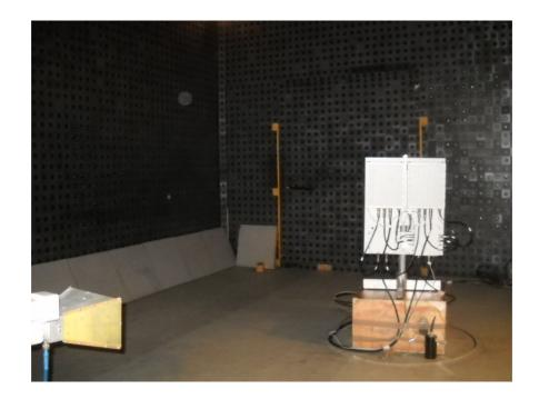
Photograph No.5 Spurious emissions measurement setup in the anechoic chamber, close view
