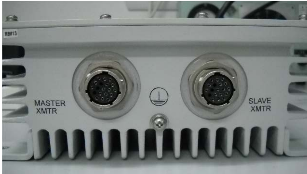
Photograph No.8 Beacon RB CLK box bottom (connectors) view
