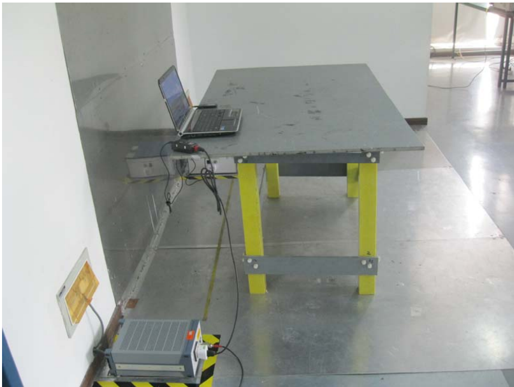
Conducted Emissions Test Setup - Side View
