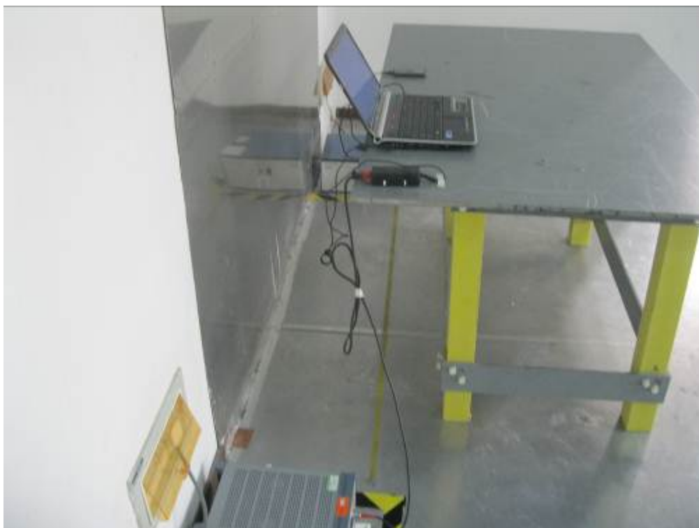
Conducted Emissions Test Setup Side View
