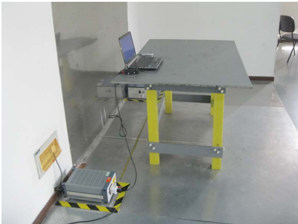
Conducted Emissions Test Setup Side View
