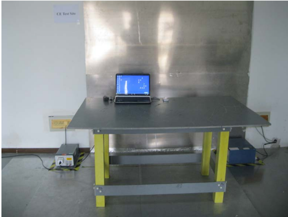
Conducted Emissions Test Setup Front View
