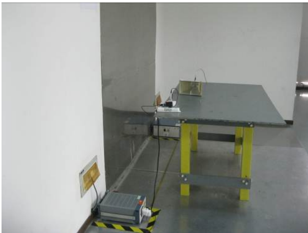
Conducted Emissions Test Setup Side View
