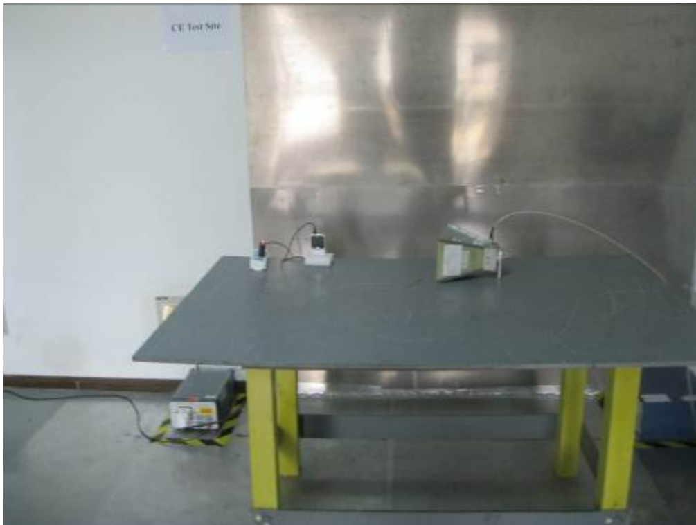
Conducted Emissions Test Setup Front View
