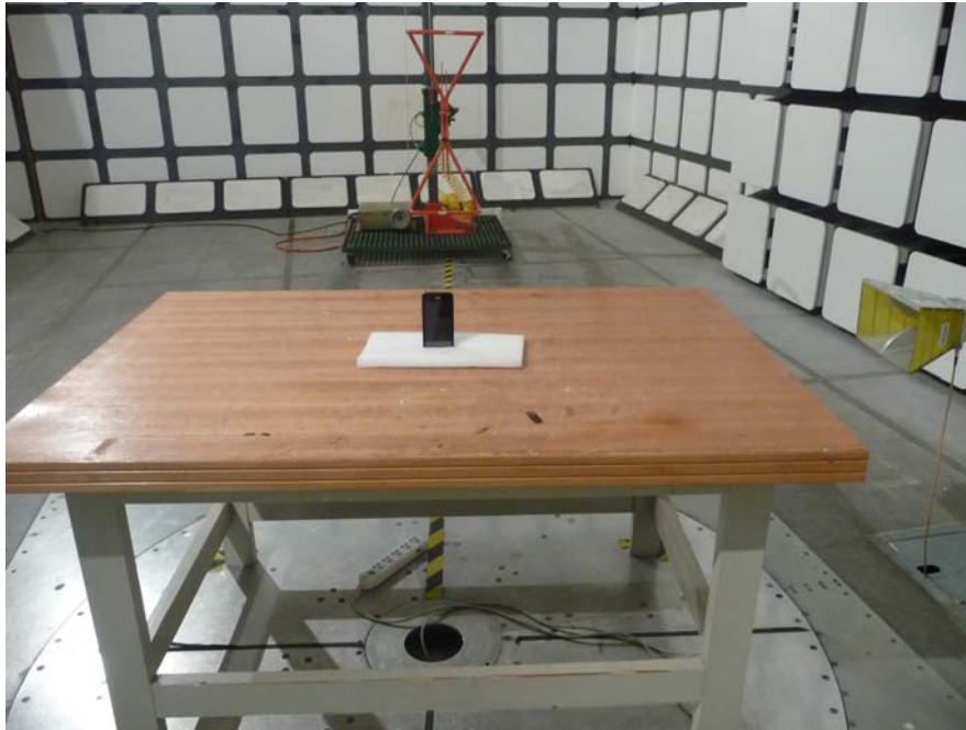
Radiated Emissions View (Below 1 GHz)
