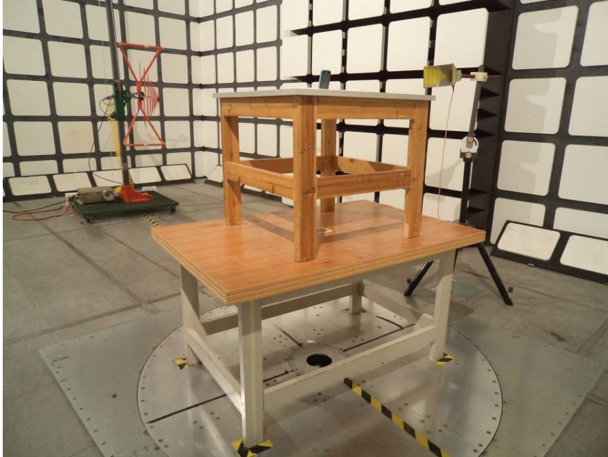
Radiated Emissions Test View (Below 1 GHz)
