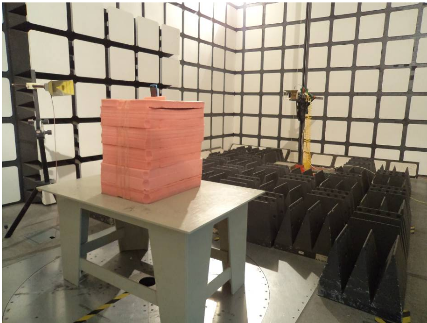
Radiated Emissions Test View (Above 1 GHz)
