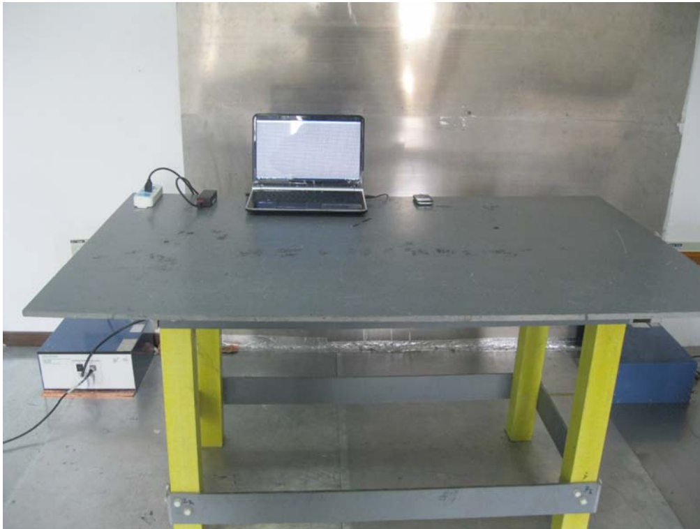
Conducted Emissions Test Setup - Front View
