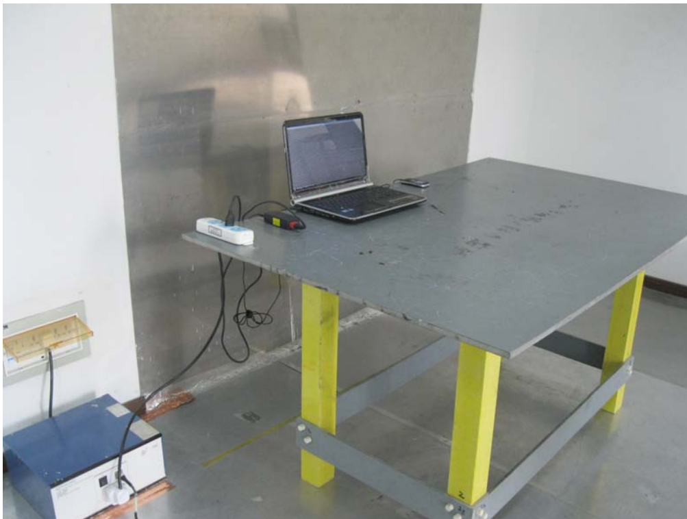
Conducted Emissions Test Setup - Side View
