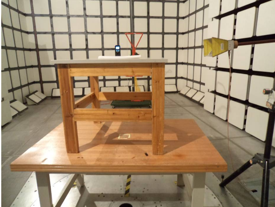
Radiated Emissions Test View (Below 1 GHz)
