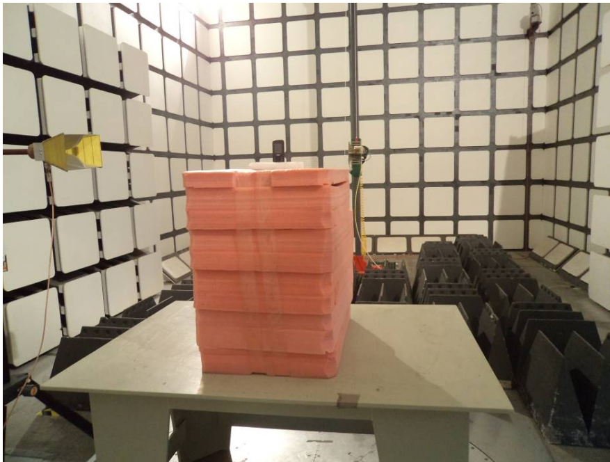
Radiated Emissions Test View (Above 1 GHz)
