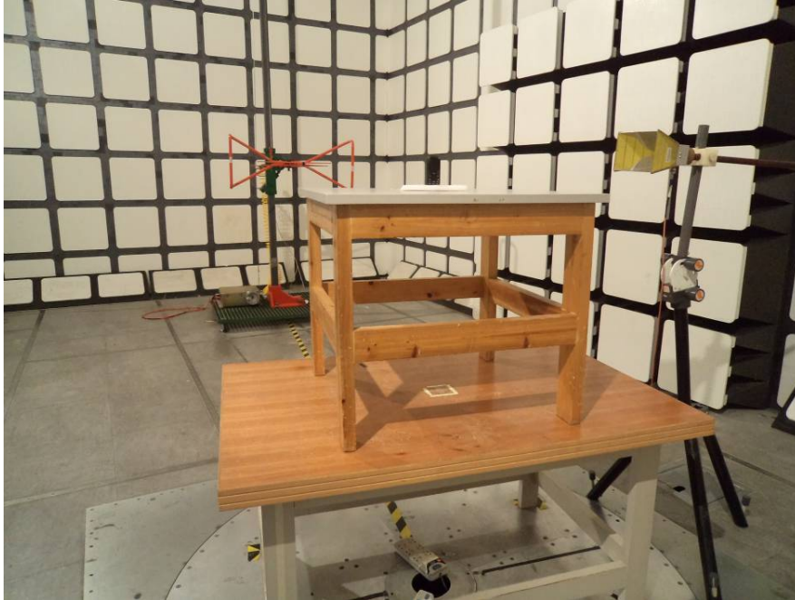
Radiated Emissions Test View (Below 1 GHz)
