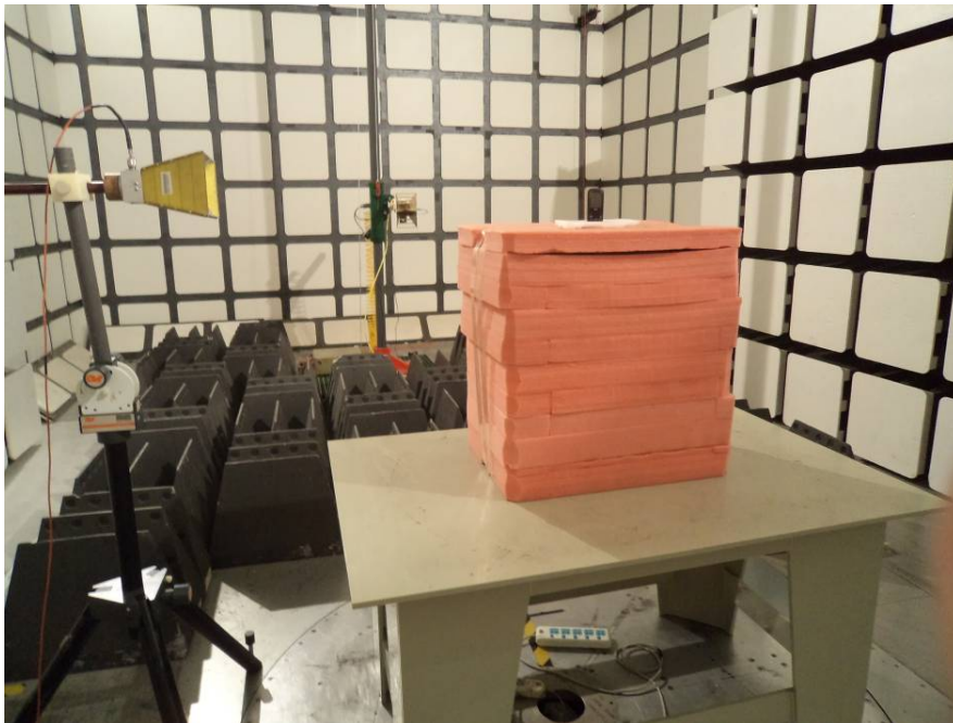
Radiated Emissions Test View (Above 1 GHz)
