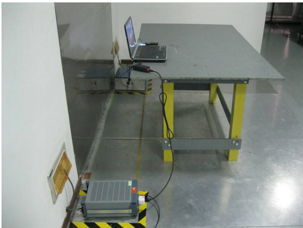
Conducted Emissions Test Setup Side View
