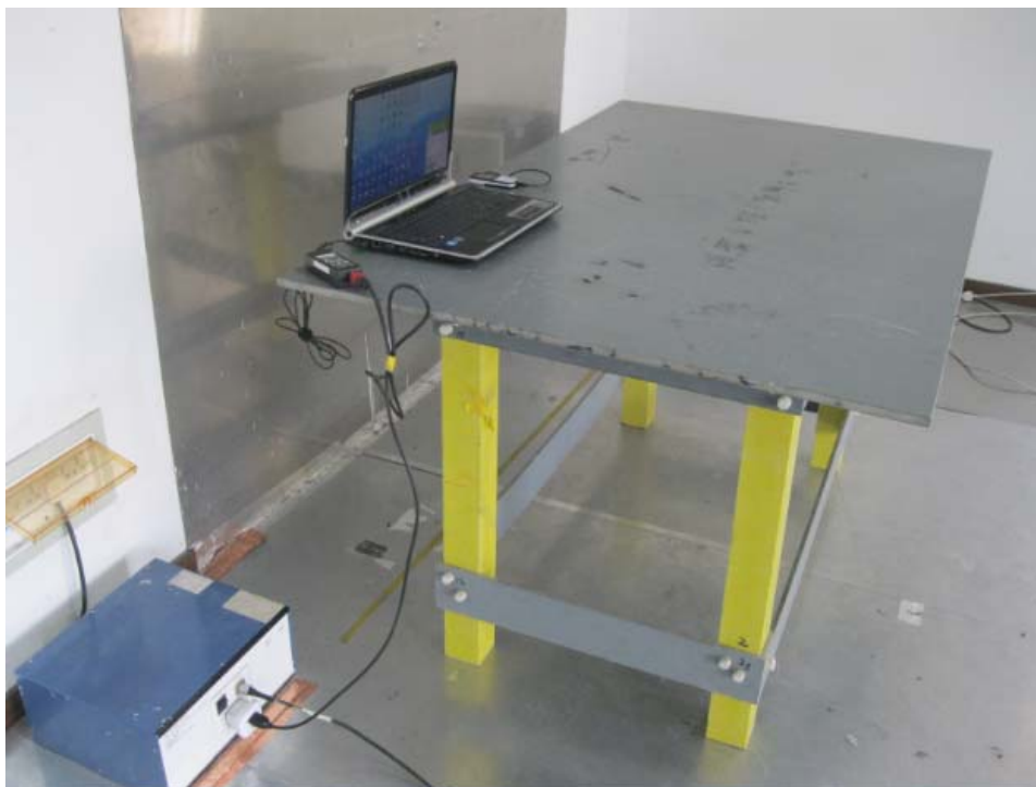
Conducted Emissions Test Setup - Side View
