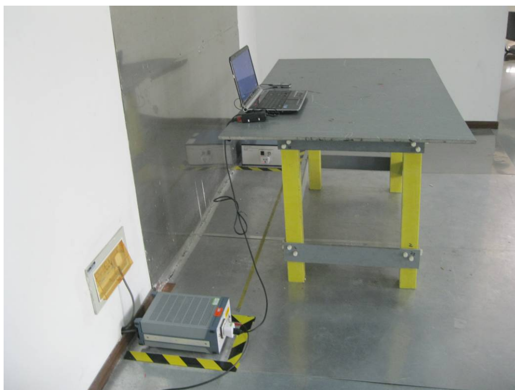
Conducted Emissions Test Setup Side View
