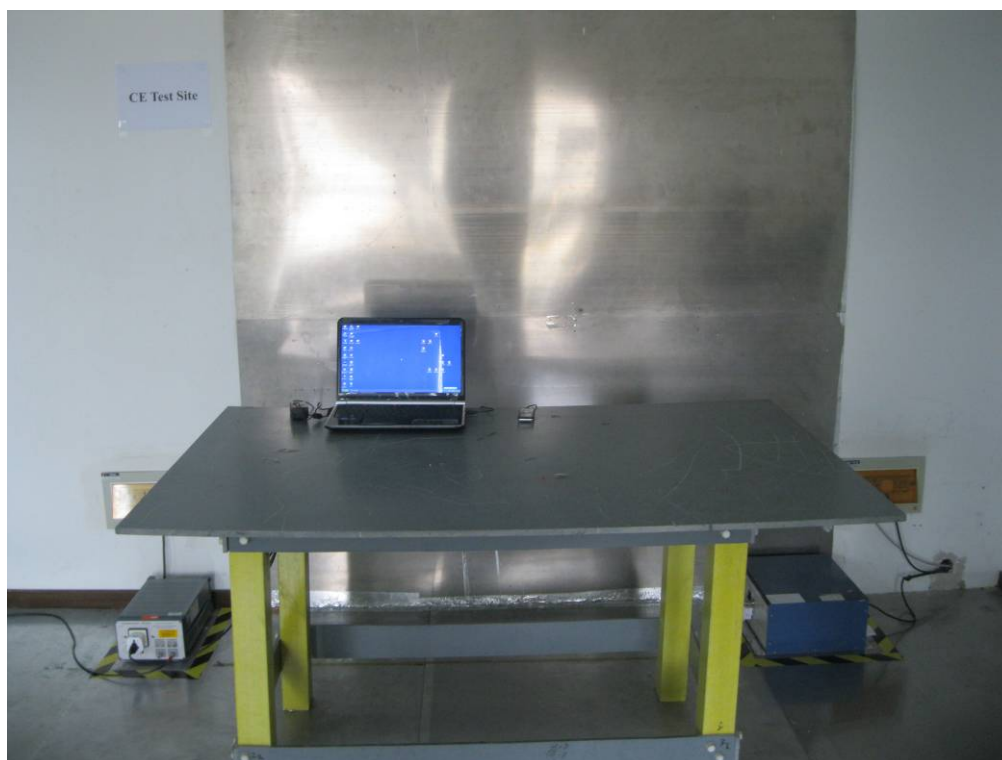
Conducted Emissions Test Setup Front View
