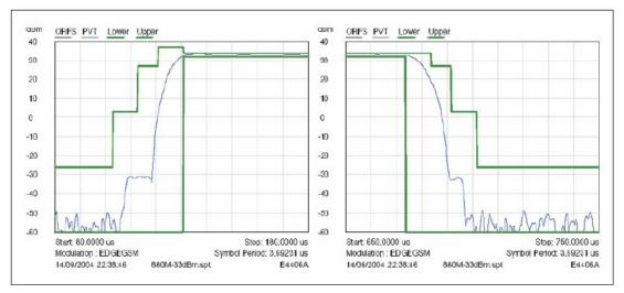
GPRS Output Power GSM850&PCS1900 allowed maximum output reduction in a multislot Configuration
